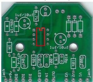
Step 4: Add the 741 single op amp. Match up the notch on the IC with the notch on the layout. If you IC does not have a notch it will have a small dot in one corner that indicates pin #1. Match up pin #1 with the square solder pad.
