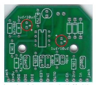
Step 7: Add the aluminum electrolytic caps. Use the 10uf for 250 specs or use the 1uf for Dist+ specs. Aluminum electrolytic capacitors are polarized. The longer lead will be the positive and should go in the square solder pad. The sorter lead will be negative. It will have "-" markings running down the side of the cap. The negative lead goes in the round solder pad.
