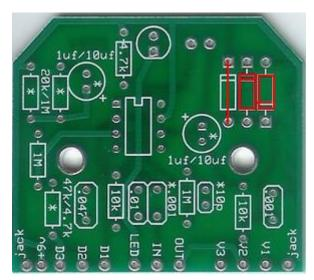
Step 3: Add the diodes. For 250 specs add the two 1N914(small orange with black stripe)with the jumper. For Dist+ specs add the two 1N34A (clear glass germanium)with the jumper. You can experiment with your own "asymmetrical" clipping by using one of the extra diodes in place of the jumper. Be sure to install the diodes in their sockets so that the stripes match up.
