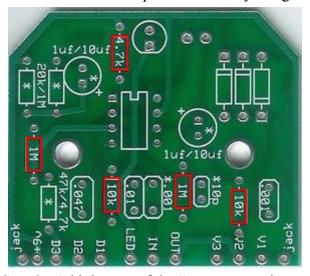
Step 2: Add the rest of the "common" resistors.
