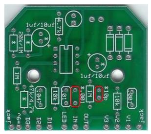
Step 5: Add the first two caps or omitt them. If you are building to 250 specs, do not add these caps. If you are building to Dist+ specs, then add them. Film and ceramic disc capacitors are not polarized so they can go in either direction.
