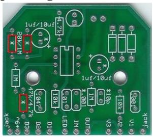
Step1: Add the first 3 resistors. Use the 20k, 20k, 47k for 250 specs or use the 1M, 1M, 4.7k for Dist+ specs. Resistors are not polarized so they can go in either direction.
