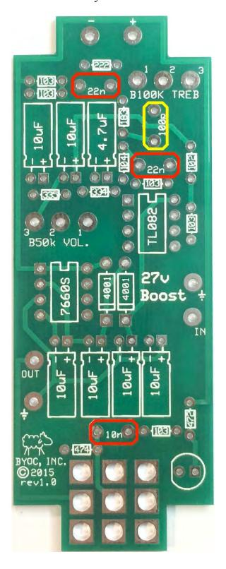
**Step** 5: Add the aluminum electrolytic capacitors. These ARE polarized, meaning there is a positive and negative end. The positive side will have a longer lead and goes in the square solder pad. The negative side will have a shorter lead and a stripe running along the body of the cap, and goes in the round solder pad. Before soldering, bend the capacitors so they lay down.
