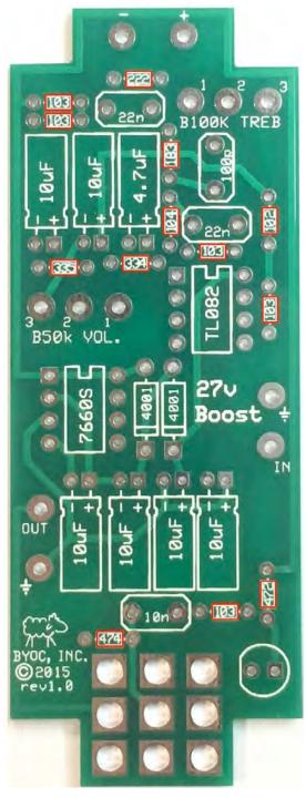
**Step 2:** Add the diodes. Be sure to match the end of the diodes with the stripe to the layout on the PCB. The striped end should go in the square solder pad.
