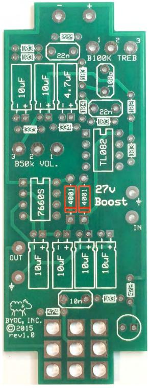
**Step** 3: Add the ICs. Be sure to orient them correctly. There may be a "U" shaped notch on the IC between pins 1 and 8. Line that up with the screenprint on the PCB. If your IC does not have a notch, look for a dot to indicate pin **1.** Pin one on the PCB will be a square hole.
