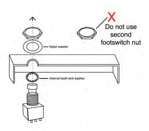
Orient the footswitch so that the flat sides of the solder lugs are like the diagram below.
