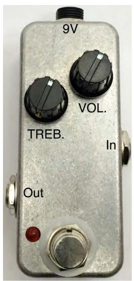
**VOL:** Adjusts the overall output volume.
