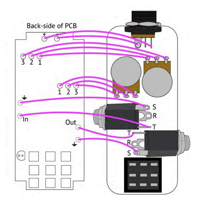
**Step 2:** Once the AC jack, potentiometers, and IN/OUT jacks are wired, insert the LED in its hole. **Insert the long lead into the square hole!!!** You might want to slightly bend the leads away from each other to keep them in the holes for now. DO NOT SOLDER YET
