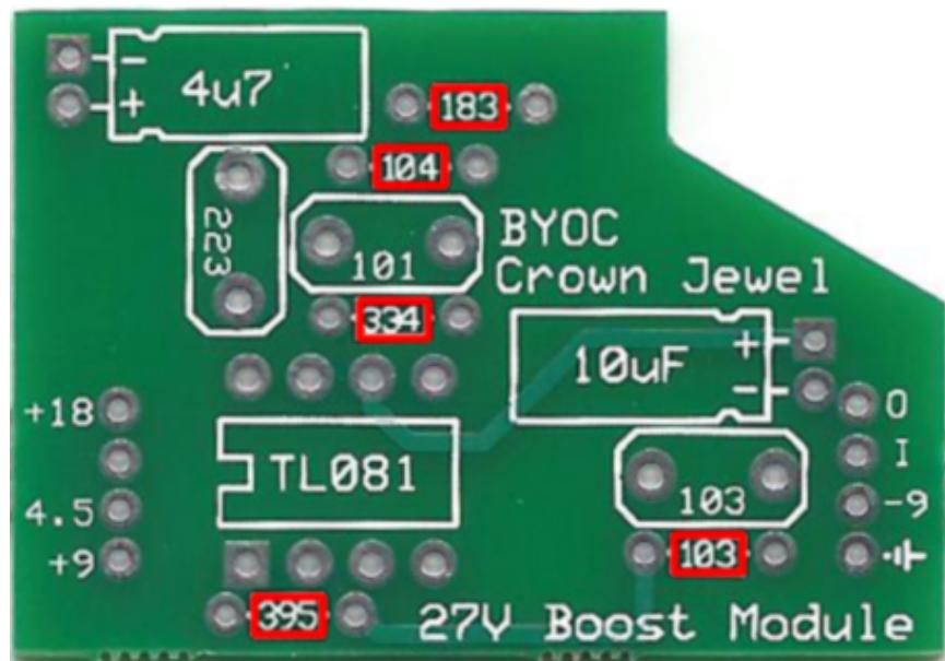
**Step 2:** Add the IC socket. Be sure to match the notch on the socket with the notch outline on the PCB screenprint.
