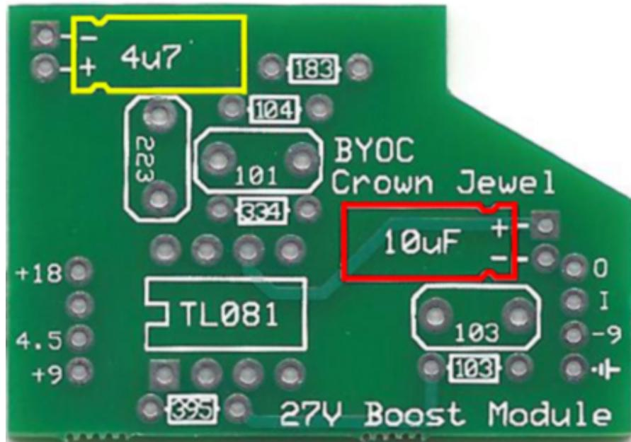
**Step 6:** Insert the pins into the Crown Jewel header spots as shown below be sure to place the longer end of the pins into the headers. Once the pins are placed, guide the module board onto the pins and press down slightly so the module is sitting flush on the pins. Solder the top-side of the module at the pins. This helps align the pins and headers to the module board.
