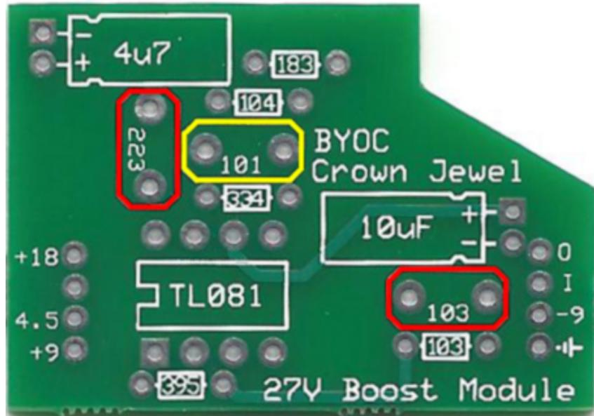
**Step 5:** Add the electrolytic capacitors. Before soldering, bend the capacitors so they lay flat along the screenprint outline. **The capacitor highlighted in yellow has a mistake on the Screenprint label. Be sure to put the long lead of the 4.7uF electrolytic into the square hole.**
