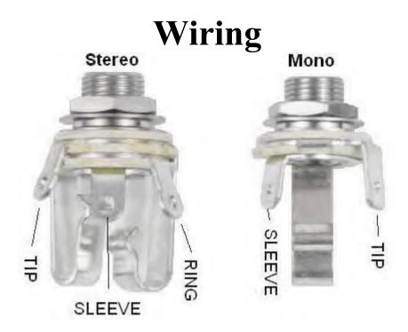
Step 1: Install the 1/4" jacks to the enclosure.
