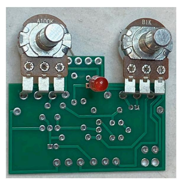
**Step 2**: Flip the PCB over so that the bottom or solder side is up. Insert the A100k (LEVEL) and B1k (FUZZ) potentiometers, and the LED into the bottom side of the PCB. DO NOT SOLDER ANYTHING YET!!! The LED will have one lead that is longer than the other. MAKE SURE THE LONGER LEAD GOES IN THE SQUARE HOLE.
