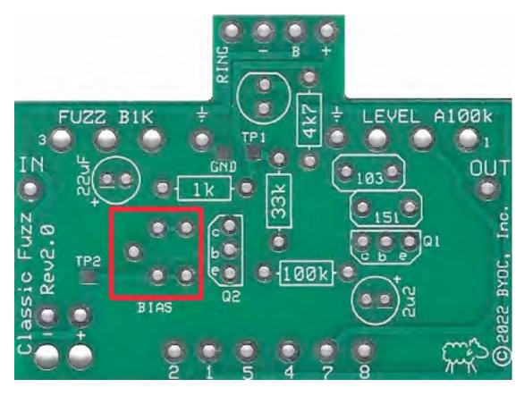
Step 5: Add the trim pot. You will notice that the space for the trim pot on the PCB has 5 eyelets, but the trim pot itself only has 3 leads. This is so that the PCB can accommodate a variety of different trim pot brands and models. There is only one way that your trim pot will be able to fit into the space in the PCB (without drastically bending the leads), so don't let this confuse you.
