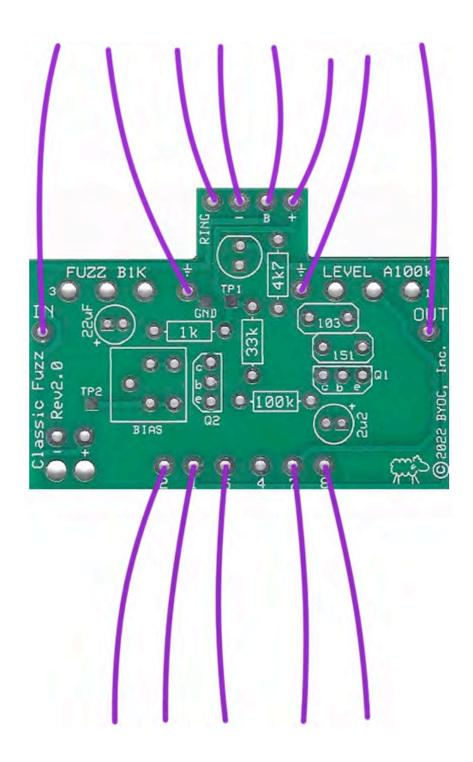
Step 8: Add the off-board wire. Add about 3" of wire to eyelets 1, 2, 5, 7, and 8. Add about 2" of wire to the IN, OUT, and two Ground eyelets. Add about 1.5" of wire to the RING, -, B, and + eyelets. This doesn't need to be exact at this point. You will trim the wire to length later.
