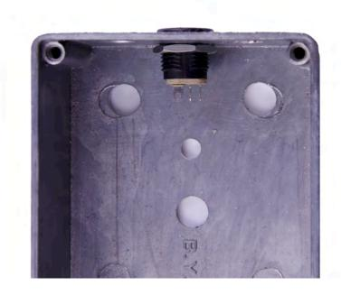
**Step 1:** Mount the DC adapter jack to the enclosure. Your kit may come with either an external thread or internal thread. Don't get confused by this. They still function exactly the same and their solder terminals will appear exactly the same. You just thread the external nut on the outside and the internal nut on the inside. The picture above is of an internal nut DC adapter jack.
