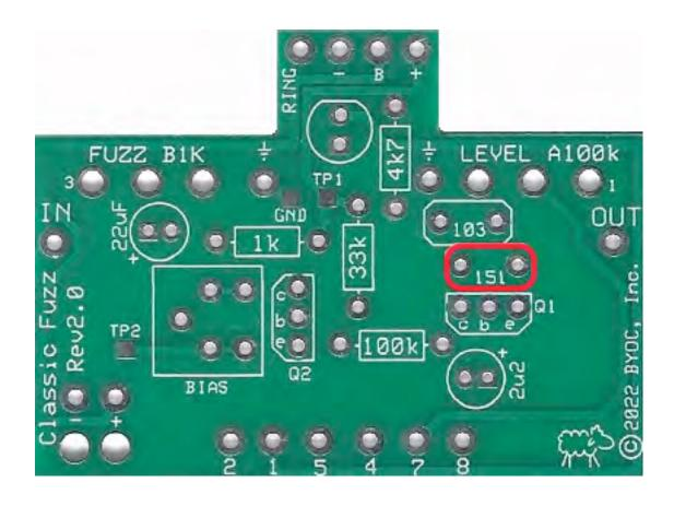
STEP 2: Add the ceramic disc capacitor. Its physical appearance may vary from batch to batch, but will most likely be a small round orange capacitor with "151" printed on the side. Ceramic disc capacitors are not polarized, so it does not matter which end goes in which solder pad.
