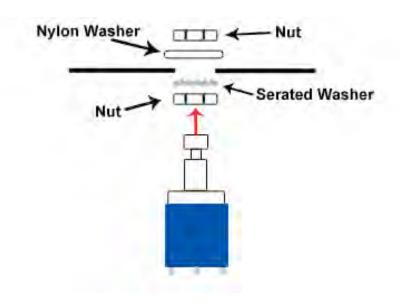
**Step 3:** Install the foot switch into the enclosure.
