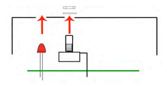
**Step 3:** Hold the PCB in one hand so that the component side of the PCB is in the palm of your hand and the bottom side with the pots, toggle switch and LED is facing up. Now use your other hand to guide the predrilled enclosure onto the PCB assembly so that the pots and LED all go into their respective holes. Once the PCB assembly is in place, secure it by screwing on the washers and nuts for the pots. Only tighten them with your fingers. You do not want them very tight yet.
