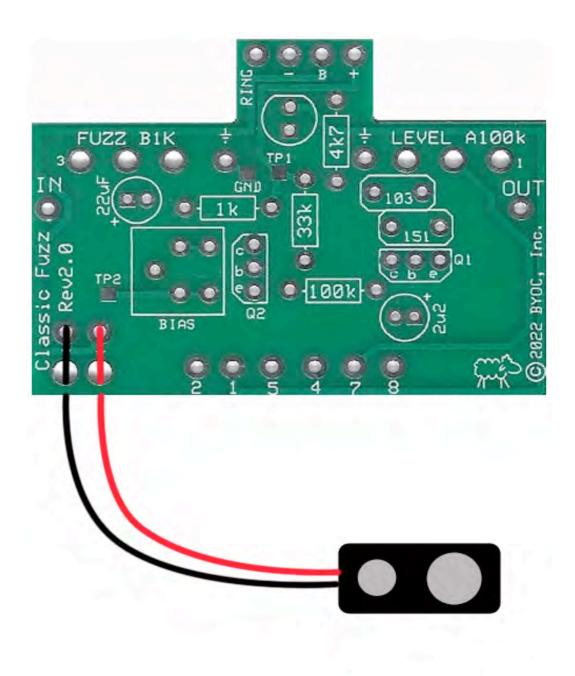
Step 7: Add the battery snap. Thread the solder ends of the battery snap into the strain relief holes from the bottom solder-side of the PCB and out through the top. Insert the solder ends of the battery snap wires into the topside of their respective solder pads. Solder on the bottom side of the PCB. Remember the red wire goes in the "+" hole and the black wire goes in the "-" hole. The supplied battery snap wires will be much longer than actually needed, so feel free to trim it to length.
