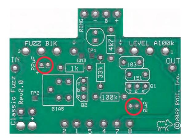
STEP 6: Add the aluminum electrolytic capacitors. **These are polarized**. The positive end will have a longer lead and should go in the square solder pad. The negative end will have a shorter lead, usually with a black or white stripe running down the body of the capacitor.
