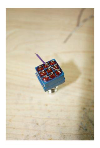
**Step 2b:** Cut a 4" piece of wire. Strip 1/2" off one end. Twist the stripped wire so that the strands are tight and then lightly tinned the exposed wire with solder. Don't use too much or it will be too thick to pass through the solder lug holes. Pass the stripped and tinned end through lug 4 and into lug 9, and then solder.
