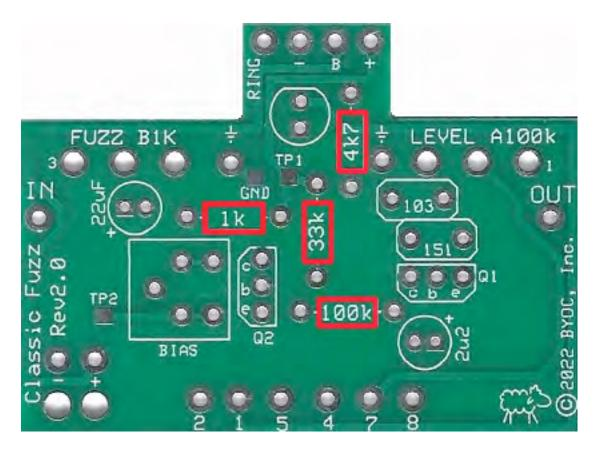
STEP 1: Add the resistors. Resistors are not polarized, so it does not matter which end goes in which solder pad. Sometimes, certain colors can be very difficult to distinguish from batch to batch. For example, sometimes the red bands in one batch may look very similar to brown. If you are having trouble differentiating color bands, it may be easier to measure the resistance using a digital multimeter.
