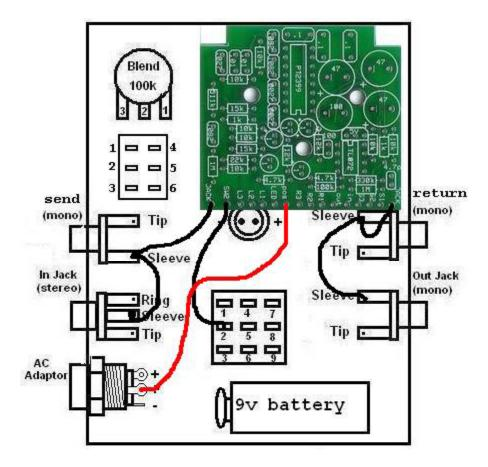
Step 14: Install the circuit board standoffs but DO NOT REMOVE the paper backings until your pedal is done and working and you are ready to close it up. You will only use 2 of the standoffs for the FX loop kit and all 3 for the base kit. Situate your circuit board inside the enclosure. For the FX loop kit the board should be to the right side over the "repeats" and "delay" knobs. For the Base kit, the board should be centered so that the standoffs mount on the back of all the pots.
