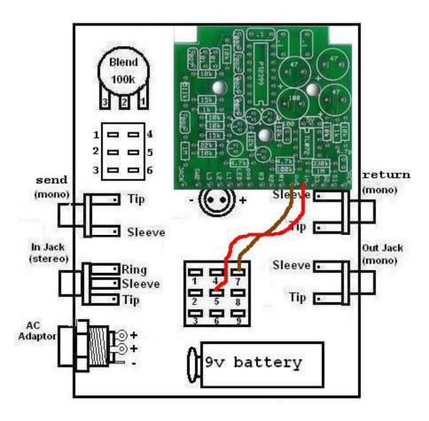
Step 18: Connect the brown wire from the "out" eyelet to lug 7 of the footswitch.
