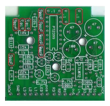
Step 7: Add the film caps. These are not polarized and can go in either direction.
