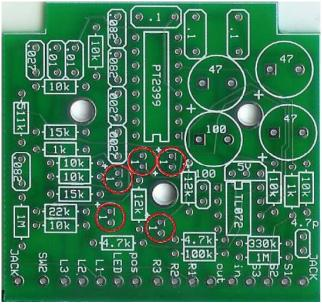
Step 3: Add all of the 1uf electrolytic caps. These are polarizes which means they have a positive and negative side. The positive side will have the longer lead and goes in the eyelet with the square solder pad. The negative side will have the shorter lead and a stripe down the side and goes in the regular round solder pad.
