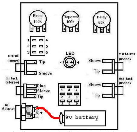
Step 8: Connect the red battery snap wire to the positive "battery" terminal of the ac adaptor jack
