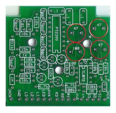
Step 6: Add the larger 100uf and 47uf electrolytic caps. These are also polarized.
