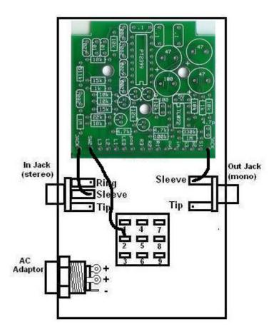
Step 17e: (FOR BASE KIT ONLY) Connect the left "jack" eyelet to the sleeve of the in jack and the right "jack" eyelet to the sleeve of the out jack.
