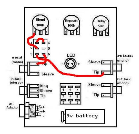
Step 9a: (FOR FX LOOP KIT ONLY) connect Lug 3 of the 100k blend pot to lug 2 of the toggle switch.
