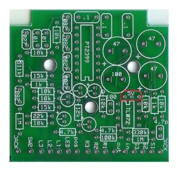
Step 4: Add the 5v voltage regulator. It will look like a plain transistor. Insert it into the board so that the flat side matches the flat side printed on the circuit board layout and the
