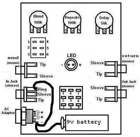
Step 6: Connect the black battery snap wire to the negative terminal of the ac adaptor jack Step 7: Connect the negative terminal of the AC adaptor jack to the ring of the in jack
