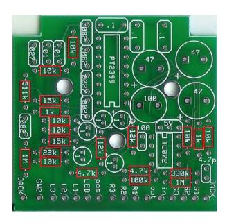
Step 1: Add all of the resistors. You will be tempted to rush this by inserting them all into the board and then soldering, but you will have much better results if you do each resistor one at a time.
