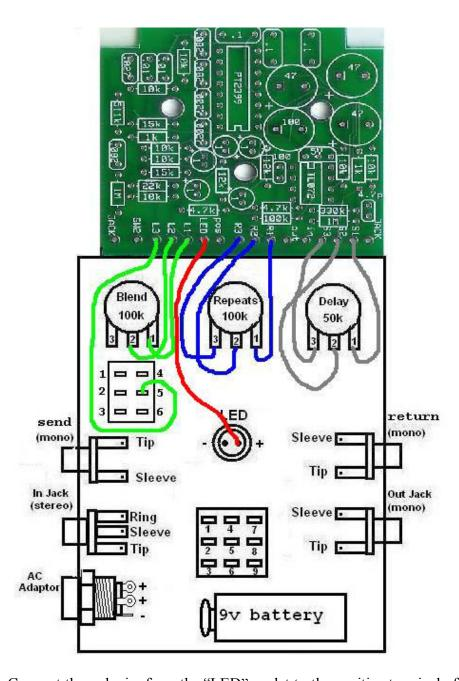
Step 10: Connect the red wire from the "LED" eyelet to the positive terminal of the LED.
