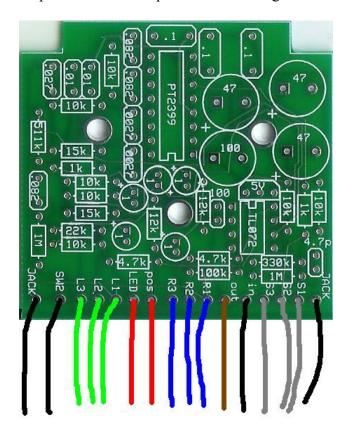
Step 8: Add the off board wires as shown above. Each wire should be about 3 inches long. NOTE the black wire from the "in" eyelet should be white. It is shown here in black for better visibility.
