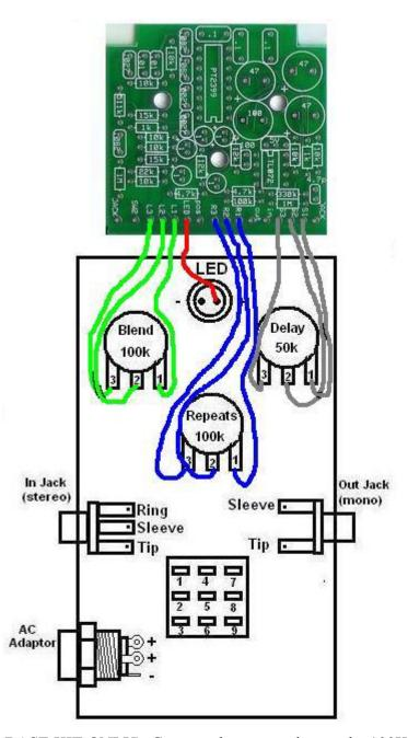
Step 13b: (FOR BASE KIT ONLY) Connect the green wires to the 100K blend pot. Connect the "L3" eyelet to lug3 of the blend pot. Connect "L2" to lug 2 and "L1" to lug 1
