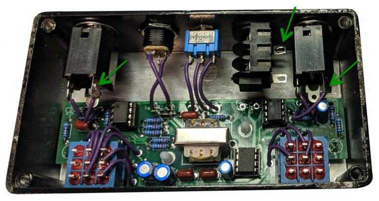
**Step 6:** Connect the wires to the respective hardware lugs. 10k 10k 10k
