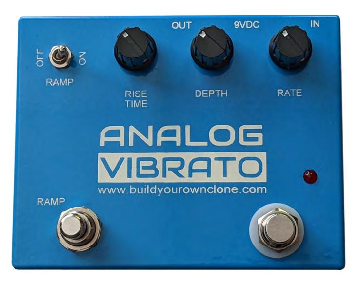
**RAMP TOGGLE:** Turns the ramp feature on or off. When the ramp is ON, use the ramp footswitch to activate the effect. When the ramp is OFF, the pedal acts as a normal vibrato.
