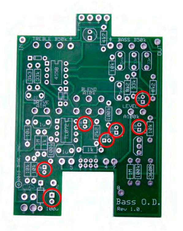
**Step 8:** Add the battery snap. Thread the solder ends of the battery snap through the strain relief holes from the bottom solder side of the PCB and out through the top. Insert the solder ends of the battery snap wires into the topside of their respective solder pads. Solder on the bottom side of the PCB. Remember the red wire goes in the "+" hole and the black wire goes in the "-" hole.
