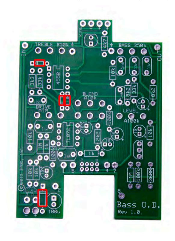
Step 3: Add 4 pin IC sockets. ONLY SOLDER THE SOCKET! NOT THE ACTUAL IC! This is a socket. The sockets get soldered to the PCB. The ICs get inserted into the sockets. The actual IC chip itself, never gets soldered. You will insert the IC into the socket after the entire pedal has been built.
