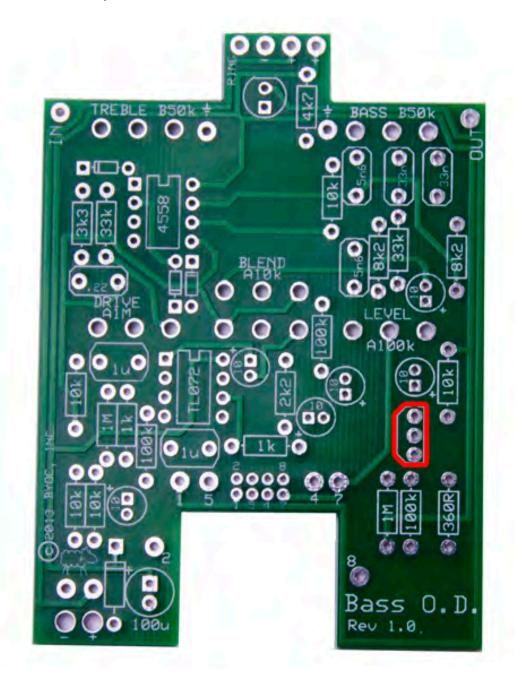
**Step 6:** Add the film capacitors. These are non-polarized so it can go in either direction. If you'd like to modify your overdrive for use with a regular 6-string guitar, use a .1uF cap in the space highlighted in green. Use a .033uf cap in the space highlighted in blue.
