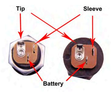
**Step 6:** Connect the TIP (negative) terminal of the DC adaptor jack to the eyelet on the PCB labeled "-". Connect the SLEEVE of the DC adaptor jack to the eyelet on the PCB labeled "+" farthest to the right. Connect the battery disconnect terminal of the DC adaptor jack to the second eyelet on the PCB labeled "+" located in the middle of the other two eyelets. See diagram on the next page.
