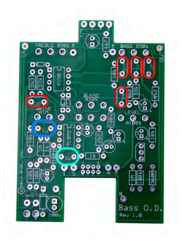
**Step 7:** Add the aluminum electrolytic capacitors. These ARE <u>polarized</u>, meaning there is a positive and negative end. The positive side will have a longer lead and goes in the square solder pad. The negative side will have a shorter lead and a stripe running along the body of the cap, and goes in the round solder pad.
