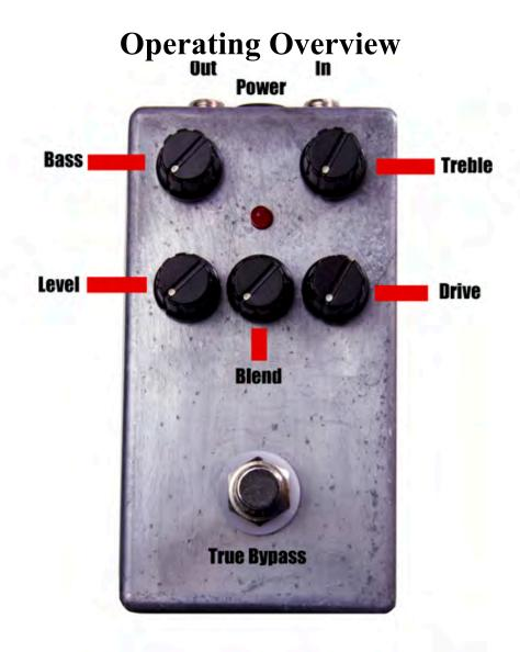
Blend: This blends your clean "dry" signal with your "wet" overdrive signal. Full turn counterclockwise is 100% dry. Full turn clockwise is 100% wet. 12 o'clock would be 50/50.
