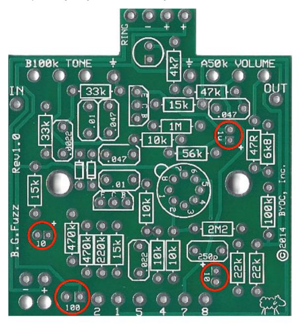
**Step 9:** Add the battery snap. Thread the leads into the strain relief holes first through the bottom side of the PCB. Then insert the leads into their respective solder pad hole on the top-side of the PCB. The red lead goes in the + hole and the black lead goes in the - hole.
