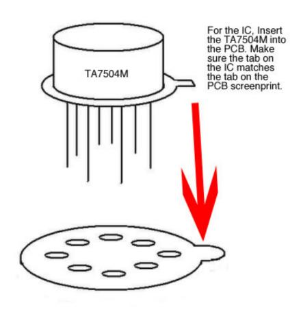
**Step 3**: Add the TA7504M IC. Be sure to align the tab on the IC with the tab outline on the PCB.
