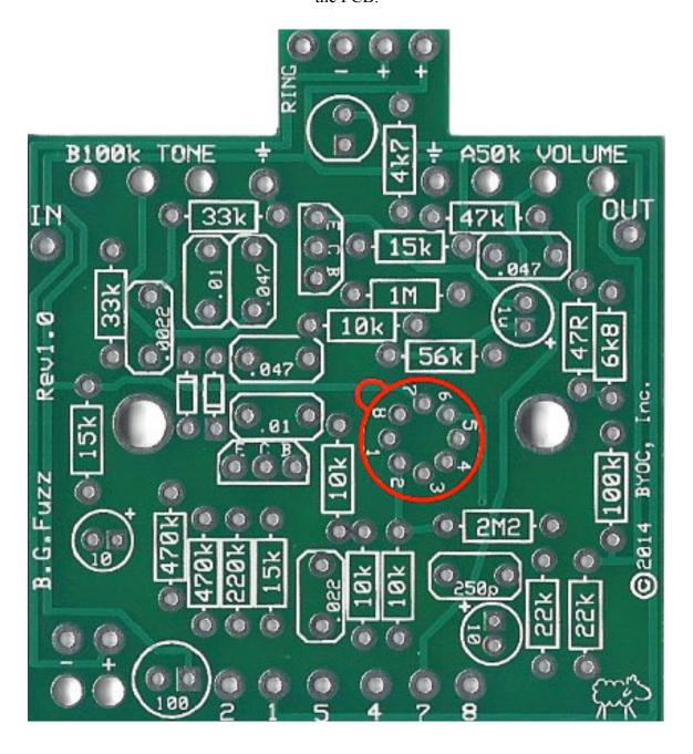
**Step5:** Add the transistors. Be sure to match the flat side of the transistor with the flat side of the transistor on PCB layout.
