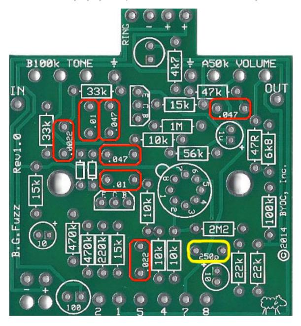
**Step 7:** Add the aluminum electrolytic capacitors. These ARE <u>polarized</u>, meaning there is a positive and negative end. <u>The positive side will have a longer lead and goes in the square solder pad</u>. The negative side will have a shorter lead and a stripe running along the body of the cap, and goes in the round solder pad.
