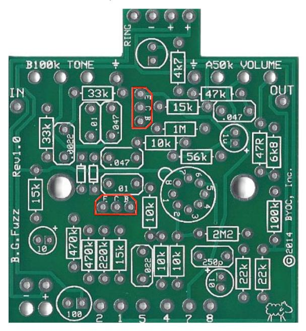
**Step 6:** Add the film capacitors. These are non-polarized so they can go in either direction. The 250p highlighted in yellow is a ceramic disc, and is also non-polarized.
