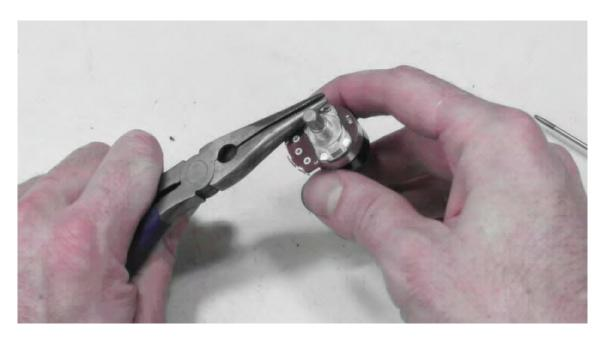
**Step 10:** Connect the other hot wire to one of the switch terminals of the Volume Potentiometer/on-off switch. This is an SPST switch, so it doesn't particularly matter which terminal you connect it to, but to avoid confusion, connect it to the terminal that is slightly more towards the right. Then use about 4" of the red cloth covered wire to connect the other switch terminal to the remaining terminal on the fuse holder.
