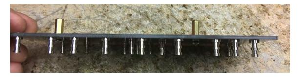
**Step 2:** Add the bare bus wire and 22k/2w resistor. The resistor is not polarized and can go on the board in either direction. Be sure to wrap these around the bottom tier of the turret lugs. Do not insert either directly into the turret lugs' shaft. Do not solder anything yet.
