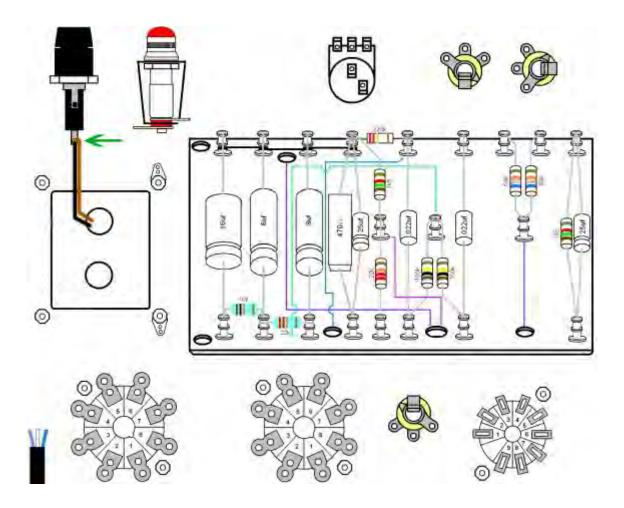
**Step 9:** Install the Volume potentiometer/ on-off switch. Snap the little node off the face of the pot first. Place the 3/8 internal lock washer between the pot and the chassis to keep it from spinning when you turn the knob. The flat washer and nut go on the outside of the chassis.
