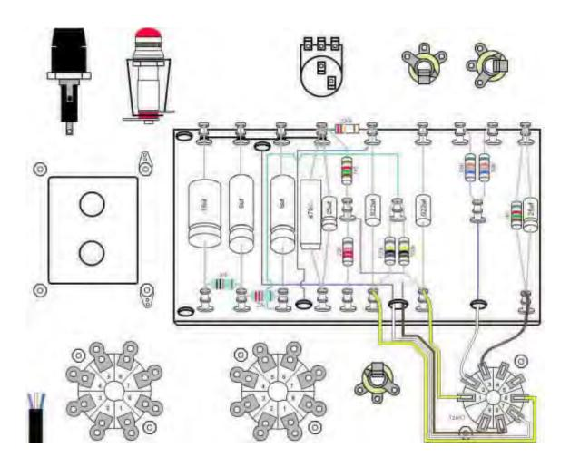
**Step 23:** Connect all but the heater wires to the 8 pin 6V6 socket. The brown wire connects to pin 8. The white wire connects to pin 5. The yellow wire connects to pin 4. The blue wire from the output transformer connects to pin 3.
