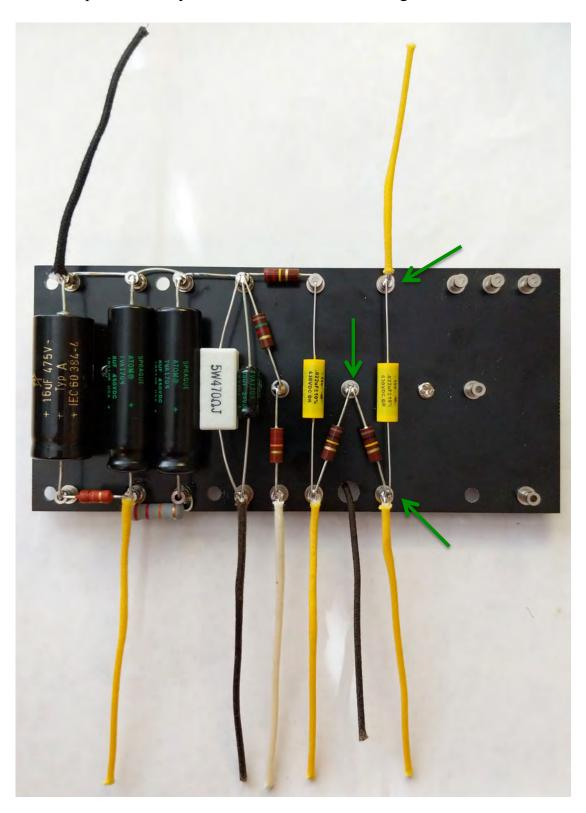
**Step 11:** Add the two 68k resistors. Insert 3" of brown wire and 3" of white wire. Solder at the green arrows.
