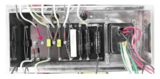
Step 2 continued: Next, very loosely screw the standoff screw into the female end of the standoff to the left between the two transformers. Then line up the holes on the right and thread the second standoff screw into the female end of the other standoff. Once you have both screws threaded into the standoffs, tighten them. Then tighten the nut that holds the standoff to the circuit board again.
