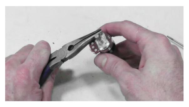
**Step 10:** Connect the black power cord wire to one of the switch terminals of the Volume Potentiometer/on-off switch. This is an SPST switch, so it doesn't particularly matter which terminal you connect it to, but to avoid confusion, connect it to the terminal that is slightly more towards the right. Then use about 4" of the red cloth covered wire to connect the other switch terminal to the remaining terminal on the fuse holder.
