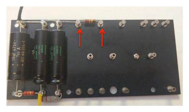
**Step 6:** Add the 470ohm/5w (10w shown in picture); 25uf capacitor; and 1k5 resistor. These components will be inserted into the tops of the turret lugs. The resistors are not polarized and can go in either direction. The capacitor is polarized and should be oriented just as the previous capacitors were. Insert 3" of brown wire into its turret lug. Now solder at the two green arrows. Be sure to solder the side of the turret lug where one end of the 220k resistor is wrapped around it.
