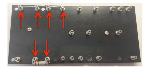
Step 3: Add the 16uf; 2 x 8uf; and 10k/2w resistor. The resistor is not polarized and can be oriented in either direction. The capacitors are polarized. It is EXTREMELY important that you orient these correctly. The positive end with be labeled with a "+" symbol. The positive end will also have an indentation around it. This end should be facing the end of the board that has the resistors. The negative end of the capacitors should be facing the end of the board that has the bare bus wire.
