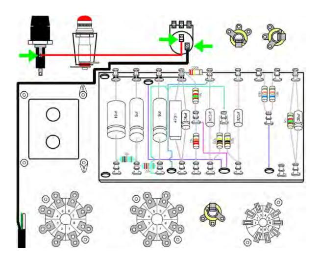
**Step 11:** Connect the white wire to the center lug of the pot. Connect the yellow wire to the lug on the right.
