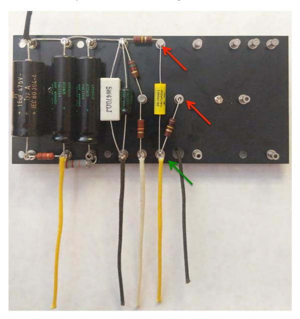
**Step 10:** Add the remaining .022uf film cap and 100k resistor. Add 2 pieces of 3" yellow wire and solder at the green arrows.
