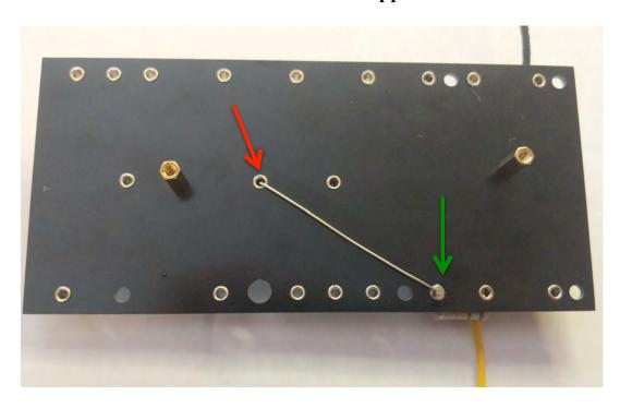
**Step 5:** Add the 220k resistor. Do not insert the ends of this resistor into the turret lug. Wrap the ends around the upper tier of the turret lugs. Do not solder yet.
