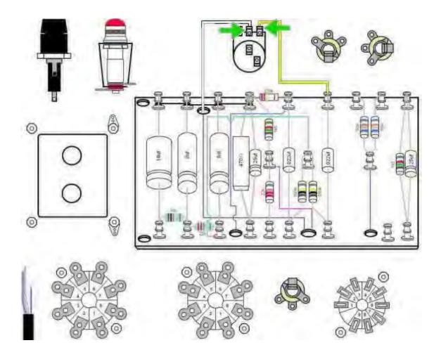
**Step 12:** Insert the black wire from the circuit board into the lug on the left. Insert a second piece of 4" black cloth covered wire into that same lug and solder both wires.
