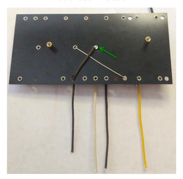
**Step 9:** Add one .022uf film capacitor and one 100k resistor. Neither of these are polarized and can be oriented in either direction. Also add 3" of yellow wire. Solder at the green arrow.
