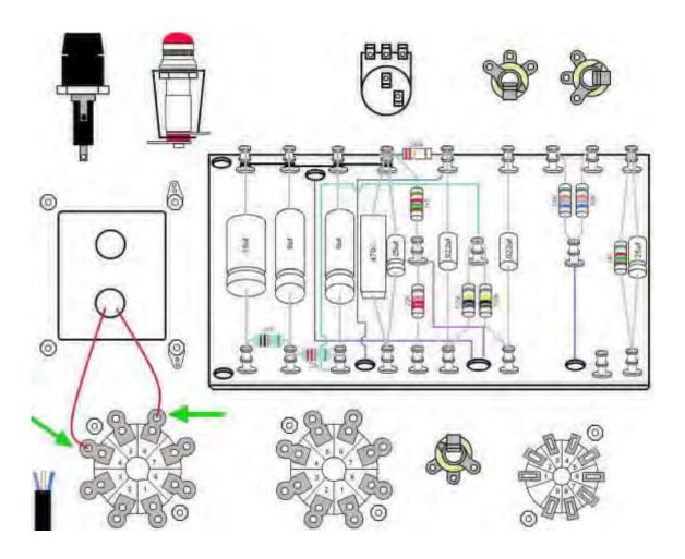
**Step 18:** Insert the red output transformer wire into the last remaining unsoldered turret lug. Strip about 1/2" off the end of the red cloth covered wire that is connected to terminal #8 of the rectifier socket and threaded through the circuit board. Wrap the stripped end of the red cloth covered wire around the bottom tier of that same turret lug. Solder the top and side of the turret lug.
