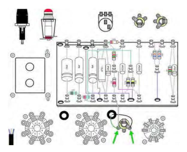
**Step 22:** Connect all but the heater wires to the 9 pin socket. You will be able to make your wiring look neater if you start with the brown wire connected to terminal #3 and work your way around the socket counter clockwise so that the last wire you connect is the yellow wire at terminal #6.
