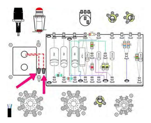
**Step 7:** Install the fuse holder into the chassis. Connect the black and brown power transformer primary wires to the solder terminal of the fuse holder that is closest to the transformer.
