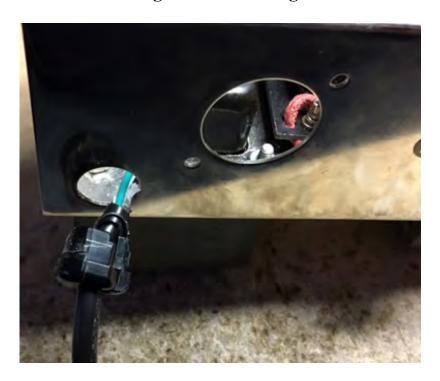
**Step 5:** Use a wire nut to connect the White wire of the power cord to black/white AND brown/white power transformer wires. Do not confuse these wires with the solid brown and solid black wires. You will want to cut these wires to an appropriate length and then strip about 1/2" off each end. Twist the wires together and then screw the wire nut on.
