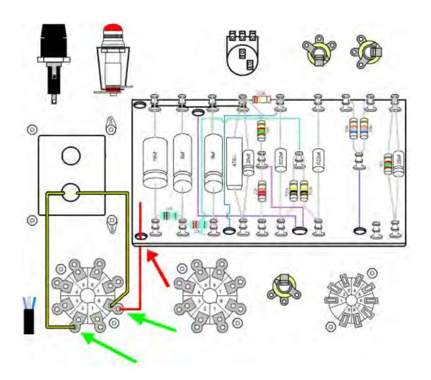
**Step 17:** Connect the secondary wires of the power transformer to the rectifier socket. One solid red wire connects to terminal #4. The other solid red wire connects to terminal #6. It does not matter which red wire goes to which terminal.
