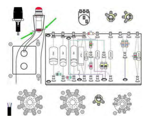
**Step 29:** Twist the two green cloth covered wires from the lamp holder together and connect them to the 8 pin 6V6 socket. Connect one wire to the inner solder hole of terminal #2 and the other wire to the inner solder hole of terminal #7. It does not matter which wire you connect to which terminal.
