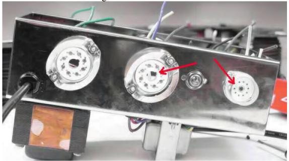
**Step 21:** Connect the speaker jack to its respective wires. The black wire from the output transformer connects to the sleeve of the jack. The green and white wires connect to the tip of the jack. The disconnect terminal of the jack is not used.
