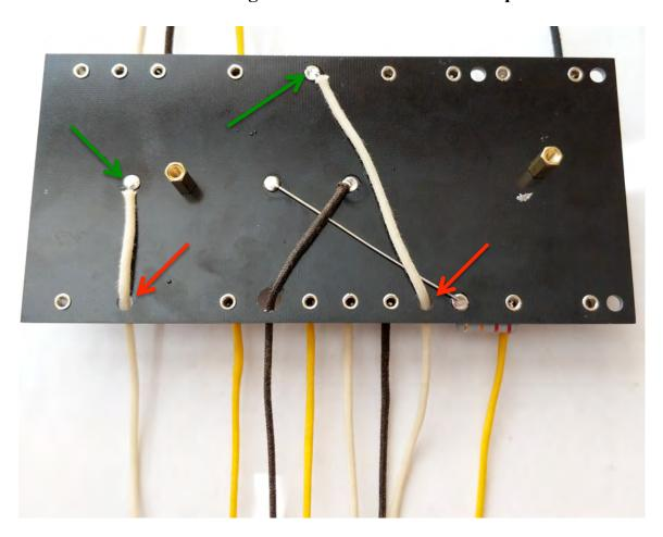
**Step 13:** Slide 8" of white wire through the two holes in the board. This wire doesn't get soldered to anything on the board, but it will get soldered to off-board components a little later.
