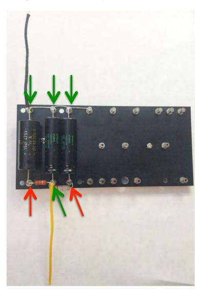
Step 4: Add bare bus wire on the underside of the board between the two eyelets shown below. Only solder at the green arrow. Be sure to flip the board over and solder the side of that same turret lug where the other end of the 22k resistor is wrapped around.
