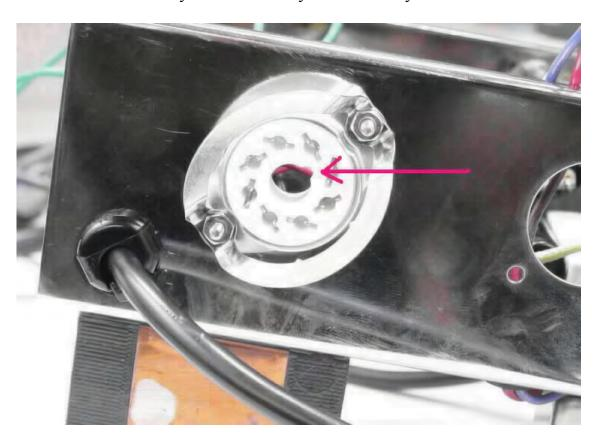
**Step 16:** Insert one of the yellow rectifier heater wires from the power transformer into solder terminal # 2 of the rectifier socket. It does not matter which yellow wire you choose. Insert the other yellow wire into terminal #8. Insert a 4" piece of red cloth covered wire into the other solder hole of terminal #8. Solder terminals #2 and #8, then thread the other end of the red wire through the hole in the circuit board.
