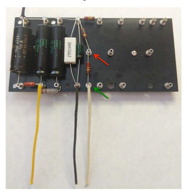
Step 8: Add 4" of brown wire on the underside of the board. Solder at the green arrow. Slide the other end of the brown wire through the hole in the board. Remember to flip the board over and solder the top-side junction of the 1k5 and 22k resistors.
