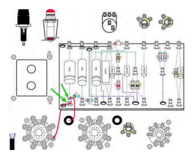
**Step 19**: Cap off the brown and yellow wires from the output transformer with the wire nuts. Fold the stripped ends of the wire over to double up the thickness of the wire so that the wire nut will catch. The brown wire is the 5K Ohm input tap. You will probably never have a need for this wire. The yellow wire is the 4 Ohm output wire.
