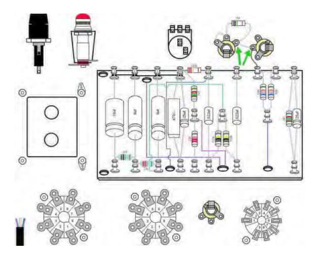
**Step 26:** Connect the black wire to the sleeve of input jack #2. Connect the white wire to the tip of input jack #2.
