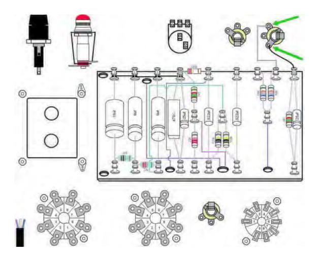
**Step 27:** Connect the solid green 6.3 VAC heater wires from the power transformer to the lamp holder. Connect one green wire to one lamp holder solder terminal and connect the other green wire to the other lamp holder solder terminal. Each terminal has two solder holes. Connect the wires to the solder holes that are closest to the center of the lamp holder. It does not matter which green wire goes to which solder terminal.
