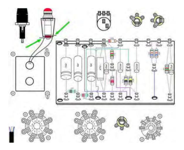
**Step 28:** Connect two 6" pieces of green cloth covered wire to the solder terminals of the lamp holder. Connect one piece to one terminal and the other piece to the other terminal. Use the outer solder holes of the terminals.
