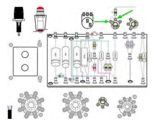
**Step 25:** Rotate the two input jacks so that the tip terminal of input jack #1 touches the disconnect terminal of input jack #2. This is what the red arrow is telling you to do before you solder anything. Thread the unsoldered end of the 1M resistor in through both these terminals. Insert the brown wire into either one of these terminals and solder them all together. It's perfectly fine if your solder forms a bridge here.
