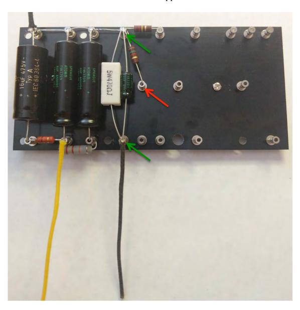
**Step 7:** Add the 1/2watt - 22k resistor and 3" of white wire. Solder only at the green arrow.
