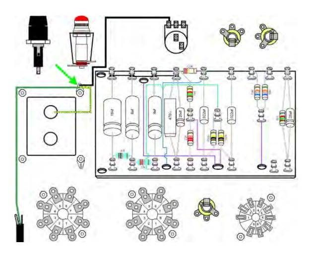
**Step 14:** Insert the red/yellow striped secondary center tap wire into the other solder terminal/lock washer and solder.
