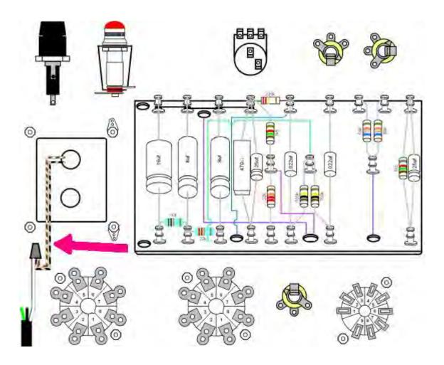
**Step 6:** Cap off the red and white striped wires of the power transformer. Do not confuse these with the red/black wire; the red/yellow wire; or the solid red wires. The red/white wires are the 550VAC secondary taps. They have a lower voltage output than the solid red secondary taps. We do not need the red/white wires. They do not get connected to anything. **DO NOT CAP THEM TOGETHER!!!** Be sure to use separate caps for each.
