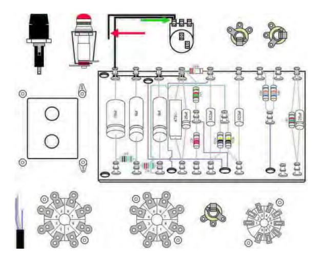
**Step 13:** Insert the other end of the black wire you just connected to the pot into the solder terminal/lock washer closest to the control side of the chassis. Insert the green/yellow striped heater ground wire and the green power cord ground wire to the solder terminal/lock washer as well. Solder all three wires to the solder terminal/lock washer.
