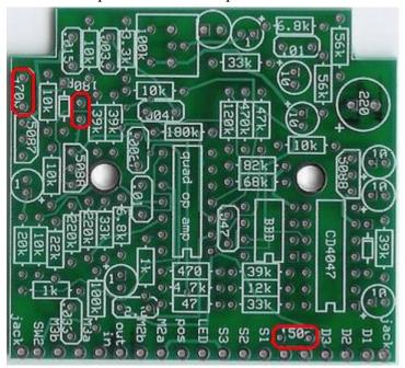
Step 9: Add the 2.2uf tantalum cap. This cap is polarized. Insert the positive end closer to the 470hm resistor and the negative end closer to the 100k resistor. Sometimes this capacitor will have a longer lead on the positive end. If both the leads are the same length, then the postive end will have a "++" symbol over the postive lead.
