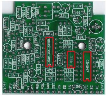
Step 4: Add the IC sockets. Do not add the actual chips themselves to the socket until the end. Make sure you line up the "u-shaped" notch in the socket to the ushaped notch on the PCB layout.
