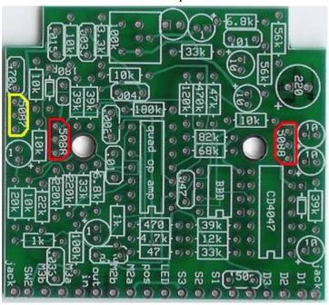
Step 7: Add the electrolytic caps. These are polarized. The positive lead will be the longer of the two and will go in the squar esolder pad.
