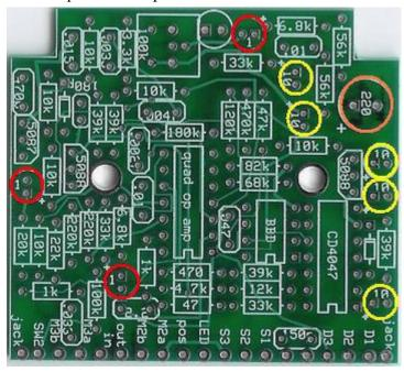
Step 8: Add the ceramic disc caps. These are not polarized.
