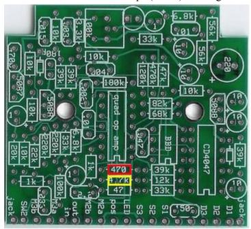
Step2: Decide if you want your LED statis light to blink or stay static. Use the 470ohm for a blinking light or 4.7k for a static light. Only add one or the other. DO NOT ADD BOTH!
