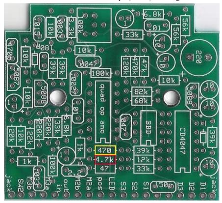
Step2: Add the LED limiting resistor. Use the 470ohm for a blinking light or 4.7k for a static light.
