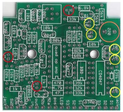
Step 8: Add the electrolytic caps. These are polarized. The positive lead will be the longer of the two and will go in the square solder pad.
