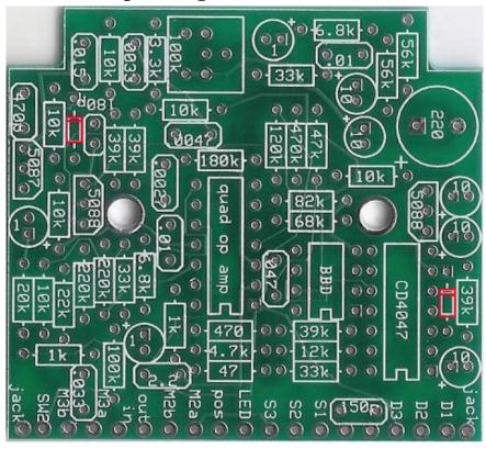
Step 1: Add the diodes. Make sure the black stripe (anode) is facing the correct way.
