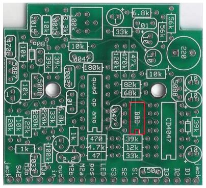
Step 5: Add the 8 pin SOCKET. Do not solder the BBD directly to the board.
