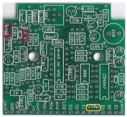
Step 9: Add the ceramic disc caps. These are not polarized.
