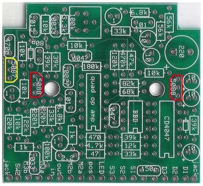
Step 7: Add the transistors. The 2N5088 are highlighted in red. The 2N5087 is highlighted in yellow. Be sure to orientate the transistors so that the flat sided match up with the circuit board layout.
