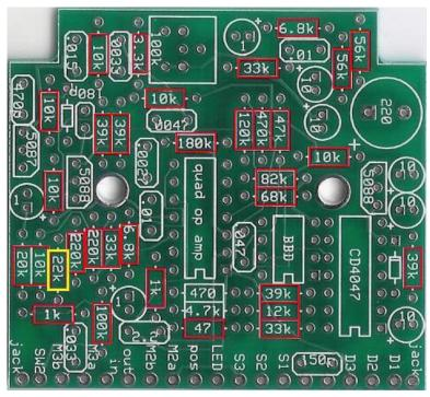
Step 3: Add the rest of the resistors. Resistors are not polarized so you can put them in either direction. You can pull the 22k resistor to modify to vibrato.
