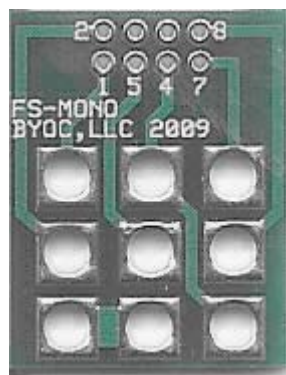
Top Side of Footswitch PCB
