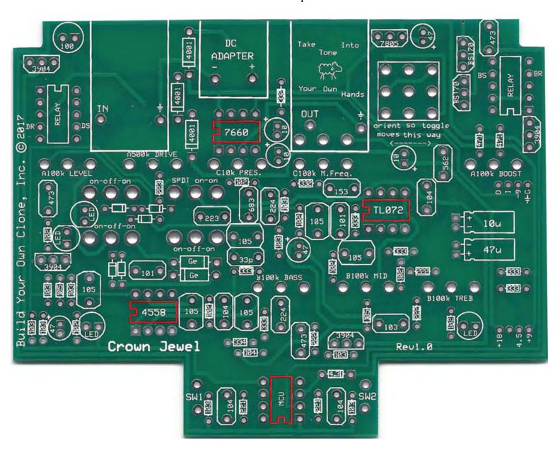
**Step 6:** Add the relays. Be sure to orient them correctly. The relay will have a line on one end of the body indicating the side where pin 1 and pin 8 are. Place the relays so the stripe side is on the notch on the PCB screenprint.
