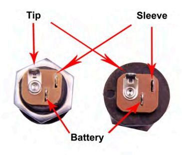
**Step 7:** Connect the TIP (negative) terminal of the DC adapter jack to the eyelet on the PCB labeled "-". Connect the SLEEVE of the DC adapter jack to the eyelet on the PCB labeled "+" farthest to the right. Also connect the enclosed audio jacks to the PCB. The SLEEVE connection will go into the ground spots, and the TIP connection will connect to the 'in' and 'out' eyelets as shown below.
