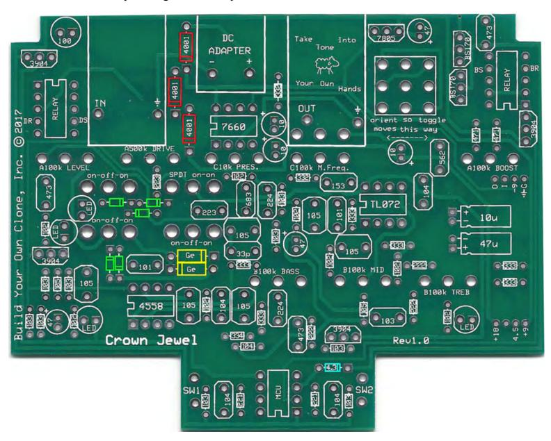
**Step 4**: Add the IC sockets. Be sure to align the notch on the IC sockets with the notch on the PCB screenprint.
