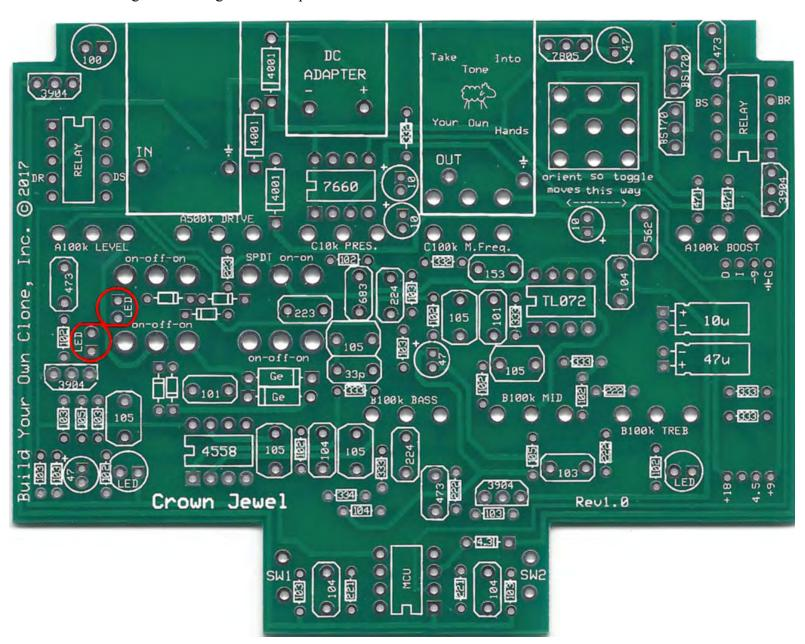
**Step 8:** Add the transistors. Be sure to match the flat side of the transistor with the flat side of the transistor on PCB layout. Red outline is 2N3904, blue outline is 78L05, and the yellow outline is for the BS170s.
