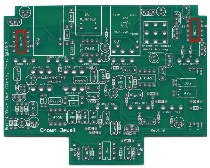
**Step 7:** Add the two clipping LEDs. Be sure to orient them according to the PCB. The longer lead will go into the square hole.
