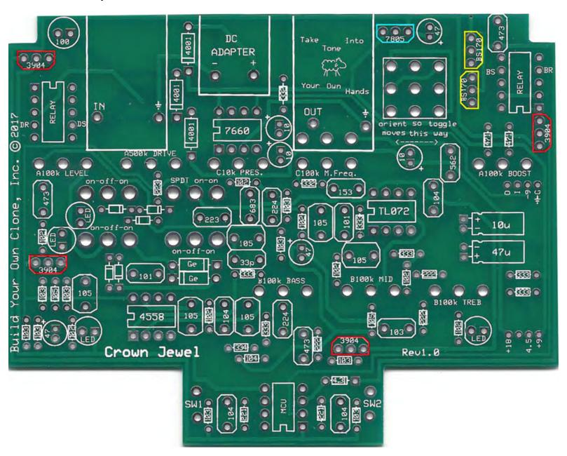
**Step 9:** Add the film and ceramic disc capacitors. These are non-polarized so they can go in either direction. The ceramic disc capacitors are highlighted in yellow, and are also non-polarized. The "473" highlighted in blue is supposed to be a .01uf film cap.
