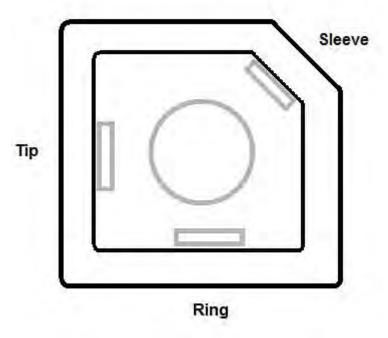
You will want to place the jacks into the enclosure so the sleeve terminal is facing the right like the picture above. Be sure to remember the lock washers so the jacks don't spin on their own.
