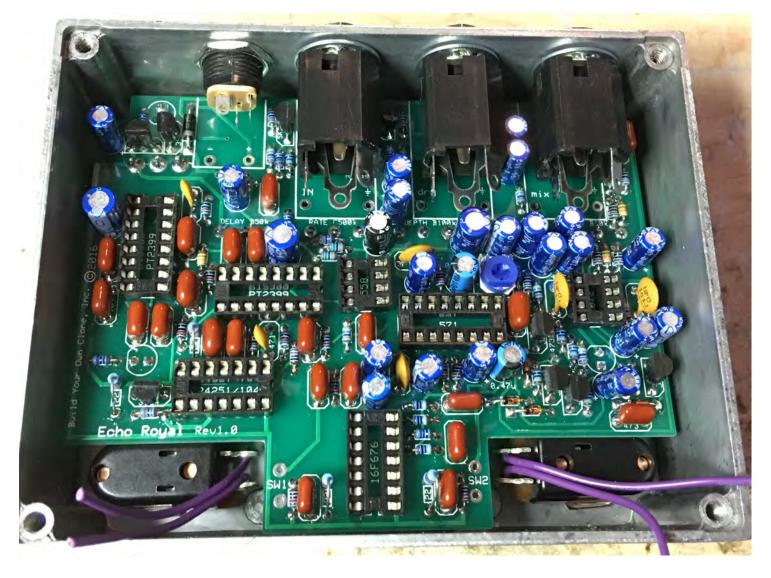
This is what your build should look like at this point. Notice the tip terminal of the AC jack is upwards, and to the left. Also note that the SLEEVE terminals of the enclosed jacks are all facing right.
