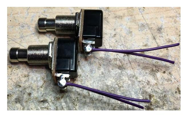
**Step 2**: Install the footswitches in the enclosure. Orient the footswitches so the solder lugs are facing each other
