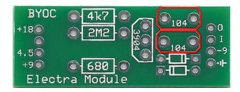
**Step 4:** Add the transistor. Be sure to match the flat side of the transistor to the flat side of the PCB screenprint.
