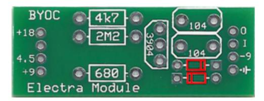
**Step 2:** Add the resistors. These are not polarized and can go in either direction.
