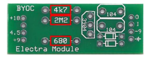
**Step 3:** Add the film capacitors. These are not polarized and can go in either direction.
