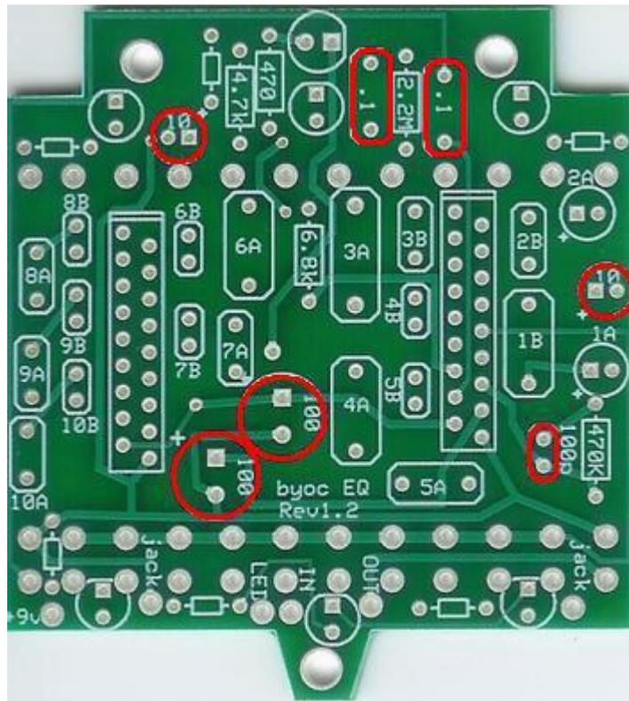
Step 3: Add the common capacitors. These are the capacitors that you will use regardless of what frequencies you want your pedal to have. The electrolytic capacitors are polarized. The longer leads go in the square solder pads. The .1uF film caps and 100pf ceramic disc cap are not polarized and can go in either direction.
