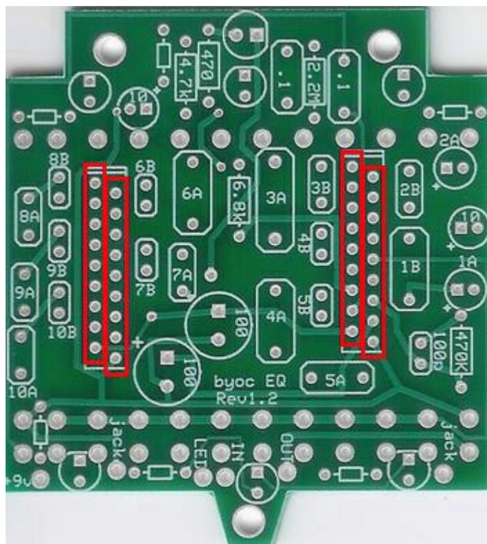
Step 4: Add the sockets for the BA3812L chips. Only solder the sockets to the PCB. Do not
