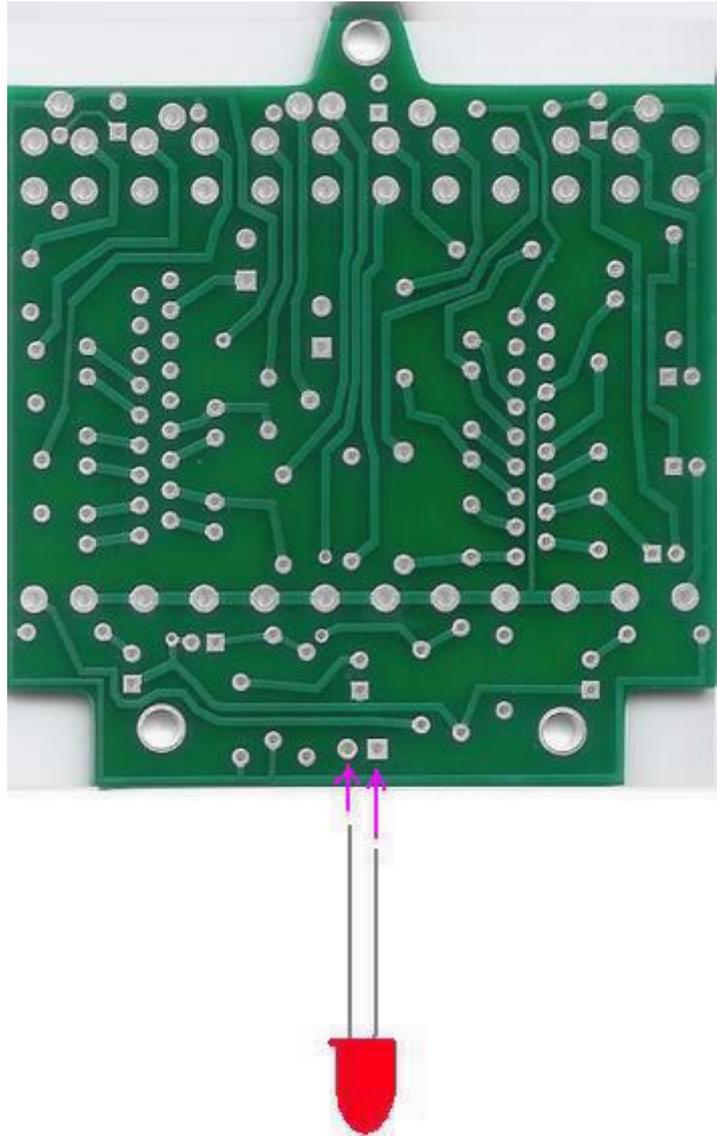
Step 4: Install the circuit board so that the 3 screws fit into the 3 mounting holes in the circuit board. CAREFULLY !!!!!!!! slide the circuit board all the way down to the nylon spacers. The slider knobs will probably not line up with their respective channels. You will need to use some sort of probe-like tool like a very small screwdriver and insert it into the trouble channels and very gently bend the entire slide to one side so that it is properly aligned with its channel.
