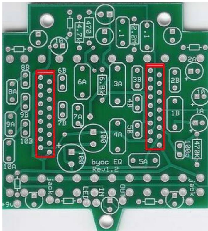
Step 7: Add the two BA3812L's. **MAKE SURE TO PROPERLY ORIENTATE THESE CHIPS!!!.** Line up the end that has the notch in it with the end of the layout that has the double lines. Make sure all the pins are straight and alligned before you try sticking it in.
