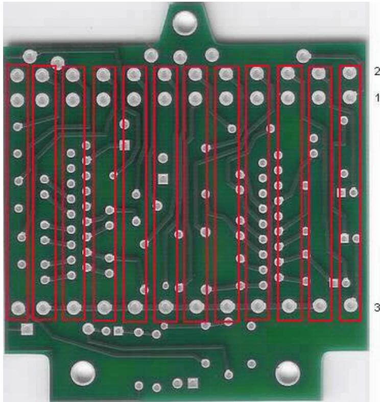
Step 6: Add the sliders. **These will go on the bottom side of the PCB.** It should be fairly obvious how to orientate them since there is only one way they can fit in the board.
