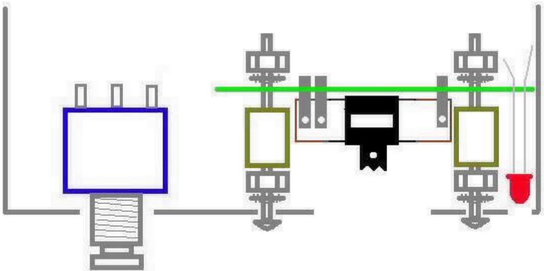
Step 1: Insert the three 4/40 screws from the outside of the enclosure. Then add one #4 toothed lock washer to each screw on the inside of the enclosure. Then add one 4/40 hex nut to each screw and tighten.
