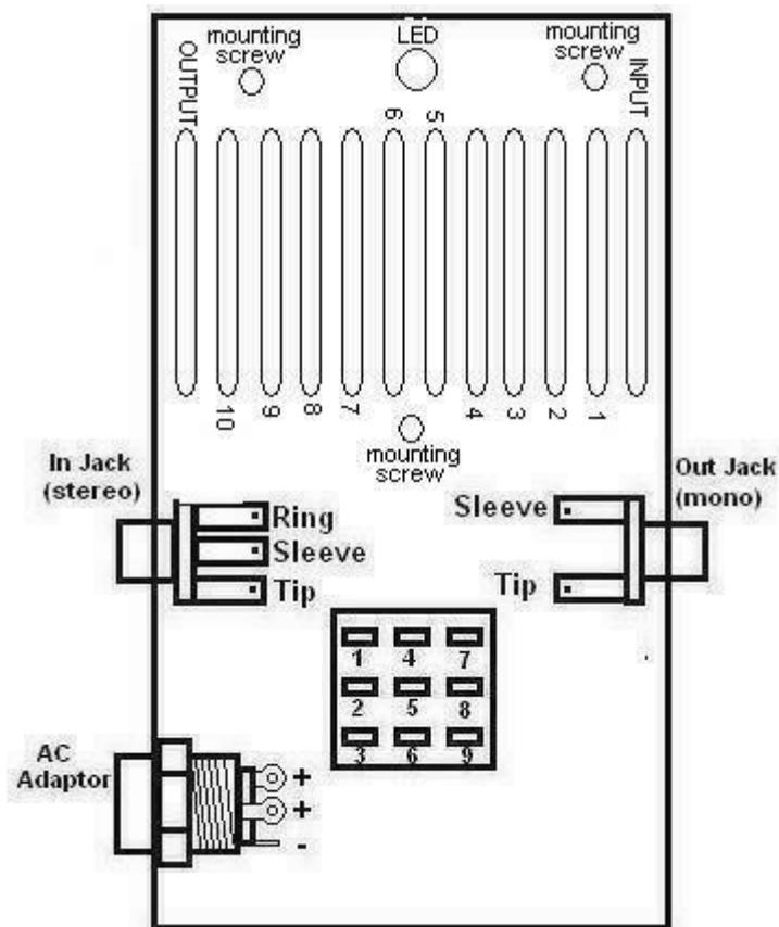
1. Install the jacks first. If you are looking down inside the enclosure, the mono jack goes on the right side and the stereo jack goes on the left. Place the washer on the outside of the enclosure. Use a 1/2" wrench to tighten.
