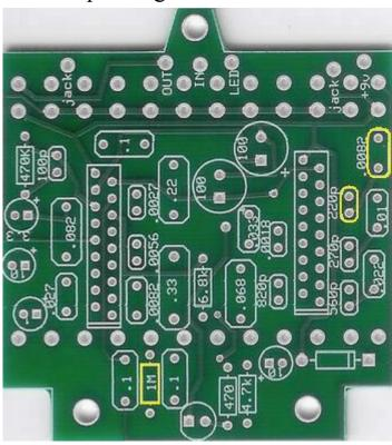
Before you start, make note that there are 3 typos on the PCB silk screening highlighted here in yellow. The 1M resistor should be a 2.2M, the 220pf cap should be a 180pf, and the .0082uf cap should be a .0068uf.
