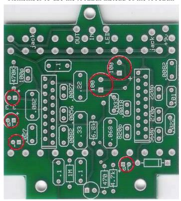
Step 5: Add the aluminum electrolytic capacitors. These are polarized. The positive lead will be longer and should go in the square solder pad. The negative lead will be shorter and have a black stripe down one side and should go in the round solder pad.
