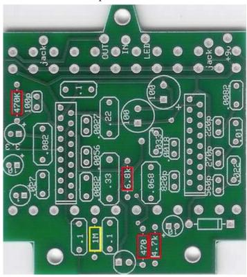
Step 1: Add the resistors. Resistors are not polarized and can go in either direction. Remember to use the 2.2m resistor in place of the 1M.
