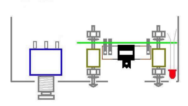
Step 1: Insert the three 4/40 screws from the outside of the enclosure. Then add one #4 toothed lock washer to each screw on the inside of the enclosure. Then add one 4/40 hex nut to each screw and tighten.
