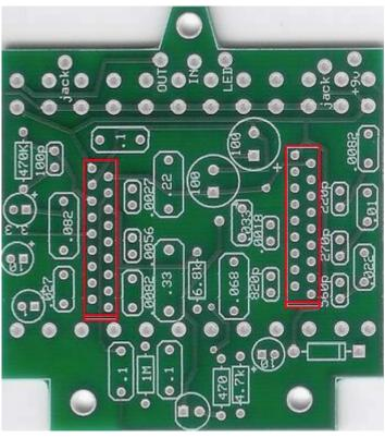
Step 6: Add the two BA3812L's. MAKE SURE TO PROPERLY ORIENTATE THESE CHIPS!!!. Line up the end that has the notch in it with the end of the layout that has the double lines. Make sure all the pins are straight and alligned before you try sticking it in.
