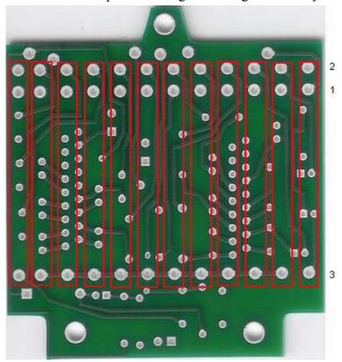
Step 7: Add the sliders. These will go on the bottom side of the PCB. It should be fairly obvious how to orientate them since there is only one way they can fit in the board.
