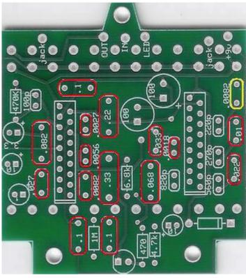
Step 4: Add the film capacitors. These are not polarized and can go in either direction. Remember to use the .0022uf instead of the .0082uf.
