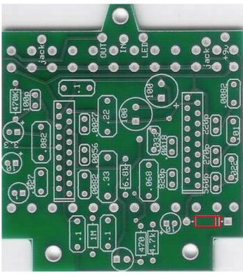
Step 2: Add the diode. Be sure to match the stripe on the diode with the stripe on the PCB layout.
