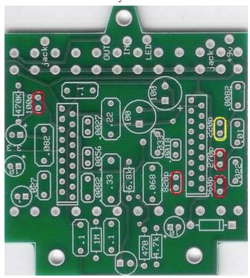
Step 3: Add the ceramic disc capacitors. These are not polarized and can go in either direction. Remember to use the 56pf instead of the 220pf.
