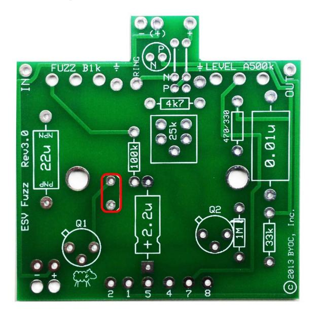
**Step 8:** Add the battery snap. Thread the solder ends of the battery snap into the strain relief holes from the bottom solder side of the PCB and out through the top. Insert the solder ends of the battery snap wires into the topside of their respective solder pads. Solder on the bottom side of the PCB. Remember the red wire goes in the "+" hole and the black wire goes in the "-" hole.
