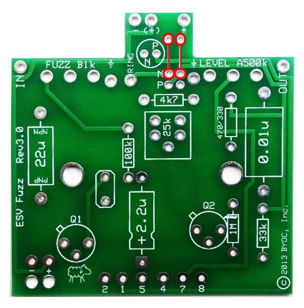
**Step 4**: Add the bias trimpot. The board is designed to accept several brands of trimmers, but there is only one way to insert the trimpot that comes with the kit. Directions for setting the trimpot are in the "Finish Up" portion of the directions.
