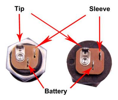
**Step 6:** Connect the TIP (negative) terminal of the DC adaptor jack to the eyelet on the PCB labeled "-". Connect the SLEEVE of the DC adaptor jack to the eyelet on the PCB labeled "+". Connect the battery disconnect terminal of the DC adaptor jack to the eyelet on the PCB labeled "(+)". See diagram on the next page.
