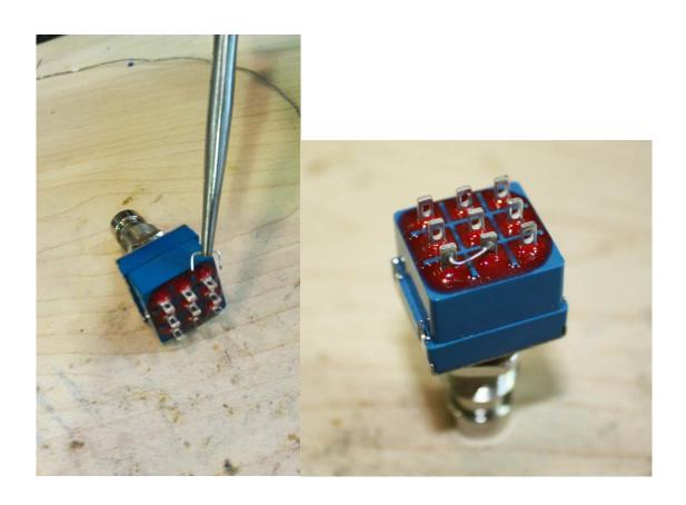
• Cut a 1.5" piece of wire. Strip 1/8" of one end. Strip 1/2" off the other end. Tin both ends. This will be used to connect lug/eyelet 4. The longer stripped end will be used to jumper lug 4 to 9.
