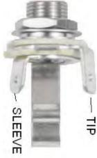
**Step 6:** Install the 1/4" jacks to the enclosure.
