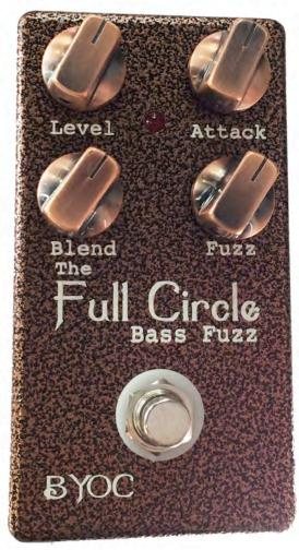
**Attack:** Sweeps between the outputs of Q2 and Q3 into Q4 to control how 'gritty' the fuzz is. Full turn clock-wise would be the Germanium transistor (Q3) and full turn counter clock-wise would be the Silicon transistor (Q2). **Level:** Controls the overall output volume.
