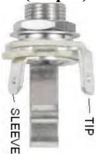
**Step 1:** Install the 1/4" jacks to the enclosure. Be sure to add the internal tooth lock washers. The lock washers go on the inside of the enclosure. The flat washers and nuts go on the outside of the enclosure.
