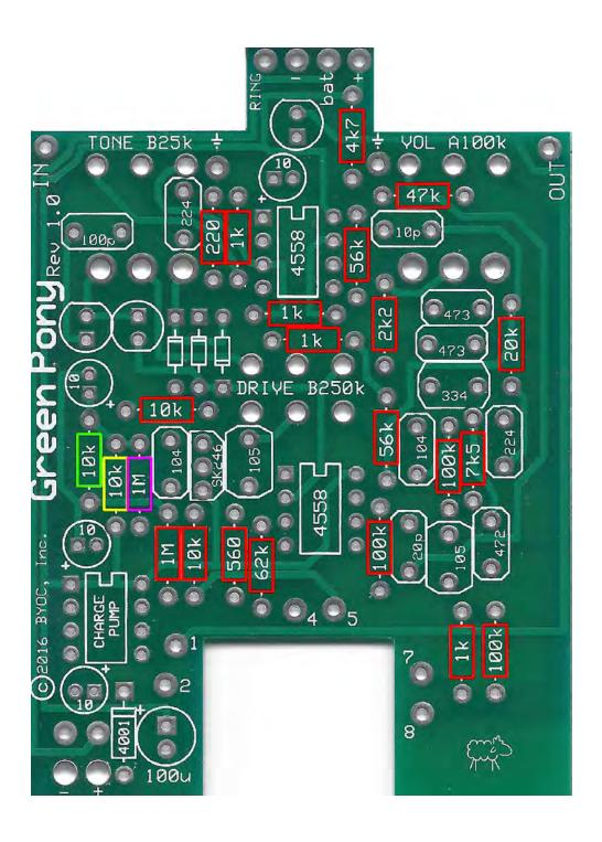
**Step 2**: Add the diodes. Be sure to match the end of the diodes with the stripe to the layout on the PCB. The striped end should go in the square solder pad. At the same time, add the two LEDs. Match up the flat side of the LED to the flat side of the screenprint. The long leg will go in the square hole.
