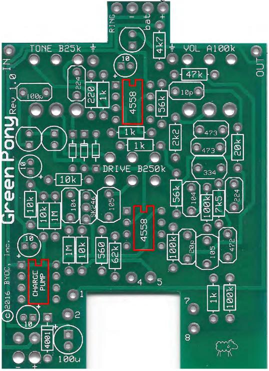
**Step 4:** Add the silicon transistor. Orient it so that the flat side matches up with the flat side on the PCB layout.
