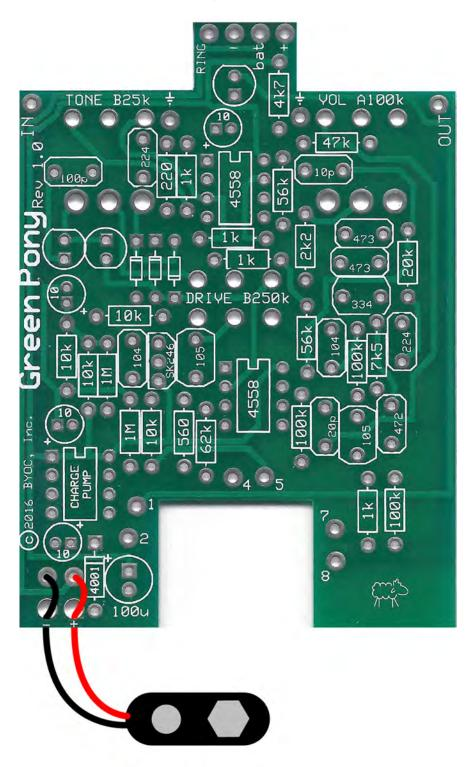
**Step 8:** Add wires to the IN, OUT, LED, POS, and the Ground eyelet located in the top of the board. Start by cutting 4 3.5" pieces of wire. Strip 1/4" off each end and tin the ends. Tinning means to apply some solder to the stripped ends of the wires. This keeps the strands from fraying and primes the wire for soldering. Load the wires in from the top and solder on the bottom of the PCB.
