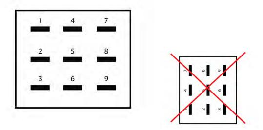
**Step 3a:** Make a jumper between lugs 3 & 6 from clippings from the resistors. Simply use your needle nose pliers to make a U shape & insert into lugs 3 & 6, then solder.
