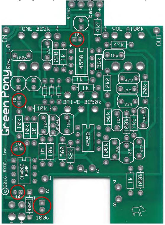
**Step 7:** Add the battery snap. Thread the leads into the strain relief holes first through the bottom side of the PCB. Then insert the leads into their respective solder pad hole on the top side of the PCB. The red lead goes in the + hole and the black lead goes in the – hole.
