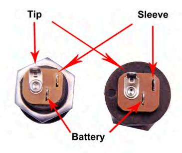
**Step 1:** Connect the TIP (negative) terminal of the DC adapter jack to the eyelet on the PCB labeled "-". Connect the SLEEVE of the DC adapter jack to the eyelet on the PCB labeled "+" farthest to the right. Connect the battery disconnect terminal of the DC adapter jack to the second eyelet on the PCB labeled "+" located in the middle of the other two eyelets .
