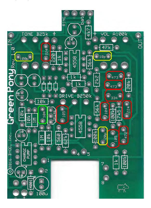
**Step 6:** Add the aluminum electrolytic capacitors. These ARE <u>polarized</u>, meaning there is a positive and negative end. The positive side will have a longer lead and goes in the square solder pad. The negative side will have a shorter lead and a stripe running along the body of the cap, and goes in the round solder pad.
