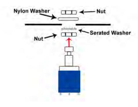
**Step 3:** Install the footswitch. Orient the footswitch so that the flat sides of the solder lugs are like the diagram below.
