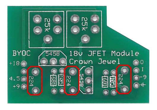
**Step 3:** Add the JFETs. Be sure to match the flat side of the JFETs to the flat side of the PCB screenprint.
