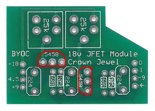
**Step 4:** Add the trimpot. There are 5 holes on the PCB, but your trimpot will only have 3 legs. This is to accommodate various styles of trimpots. Your trimpot will only orient in one direction.
