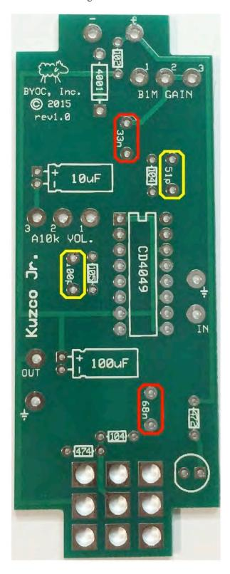
**Step 5:** Add the aluminum electrolytic capacitors. These ARE <u>polarized</u>, meaning there is a positive and negative end. The positive side will have a longer lead and goes in the square solder pad. The negative side will have a shorter lead and a stripe running along the body of the cap, and goes in the round solder pad. Before soldering, bend the capacitor so it is laying down like below
