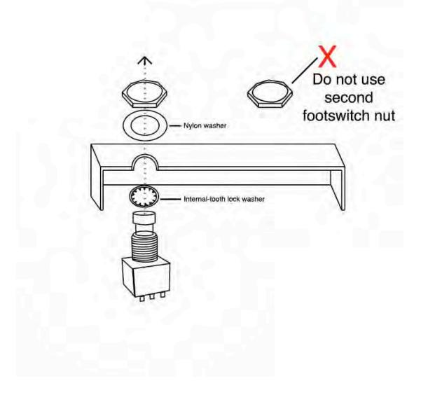
Orient the footswitch so that the flat sides of the solder lugs are like the diagram below.
