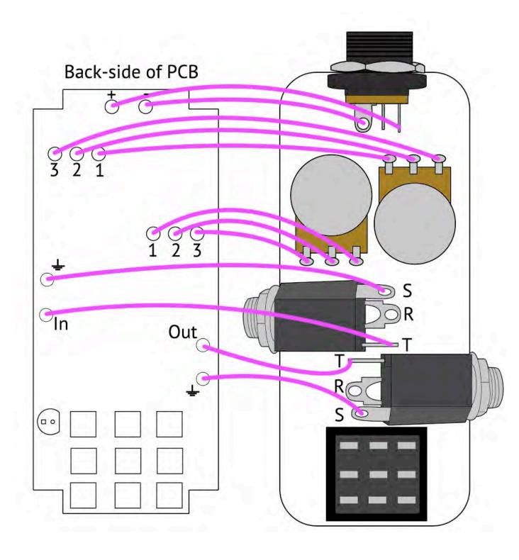
**Step 2:** Once the AC jack, potentiometers, and IN/OUT jacks are wired, insert the LED in its hole. **Insert the long lead into the square hole!!!** You might want to slightly bend the leads away from each other to keep them in the holes for now. DO NOT SOLDER YET
