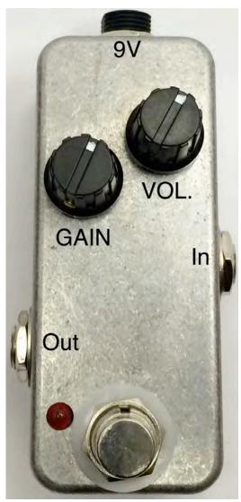
**VOL:** Adjusts the overall output volume **GAIN:** Adjust the amount of distortion **Power supply:** 2.1mm negative tip.
