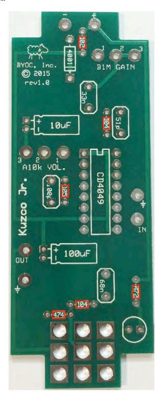
**Step 2:** Add the diode. Be sure to match the end of the diode with the stripe to the layout on the PCB. The striped end should go in the square solder pad.
