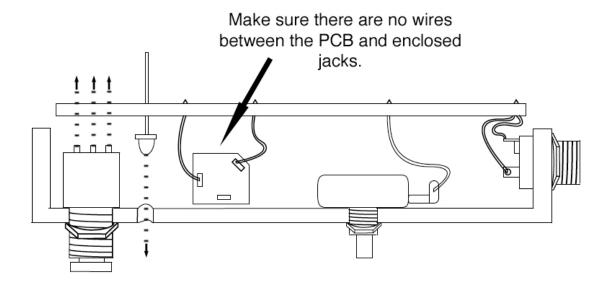
It is extremely important that when you place the PCB on the footswitch, you make sure to tuck all the wires out of the way so that that PCB can rest flush against the enclosed jacks and footswitch.
