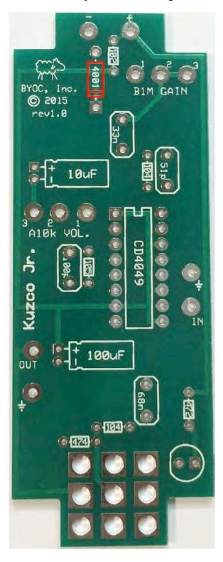
**Step** 3: Add the IC. Be sure to orient it correctly. There may be a notch on the IC between pins 1 and 8. Line that up with the screenprint on the PCB. If your IC does not have a notch, look for a dot to indicate pin 1. Pin one on the PCB will be a square hole.
