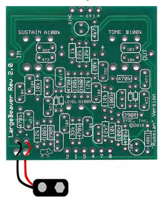
**Step 6:** Add wires to the IN, OUT, LED, POS, and the Ground eyelet located in the top of the board. Start by cutting 4 3.5" pieces of wire. Strip 1/4" off each end and tin the ends. Tinning means to apply some solder to the stripped ends of the wires. This keeps the strands from fraying and primes the wire for soldering. Load the wires in from the top and solder on the bottom of the PCB.
