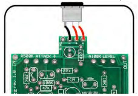
**Step 2:** Wire the PCB to the foot switch and jacks as shown.
