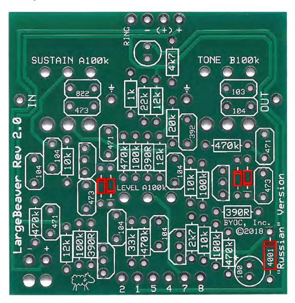
**Step 2**: Add the transistors. Orient them so that the flat side on the transistors matches up with the flat side on the PCB layout.
