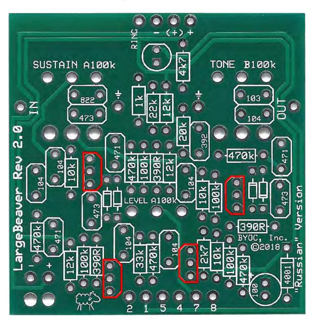
**Step 3:** Add the film and ceramic disc capacitors. These are not polarized and can go in either orientation. The capacitors highlighted in yellow are the ceramic disc capacitors.
