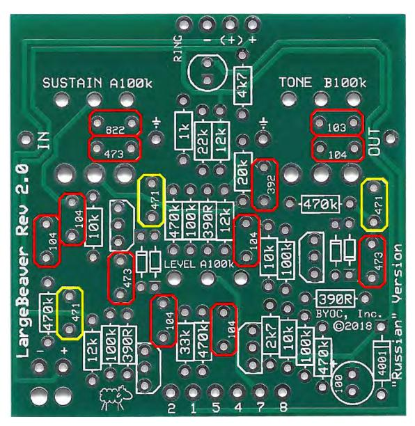
**Step 4:** Add the aluminum electrolytic capacitor. These ARE <u>polarized</u>, meaning there is a positive and negative end. The positive side will have a longer lead and goes in the square solder pad. The negative side will have a shorter lead and a stripe running along the body of the cap, and goes in the round solder pad
