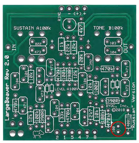
**Step 5:** Add the battery snap. Thread the leads into the strain relief holes first through the bottom side of the PCB. Then insert the leads into their respective solder pad hole on the top side of the PCB. The red lead goes in the + hole and the black lead goes in the – hole.
