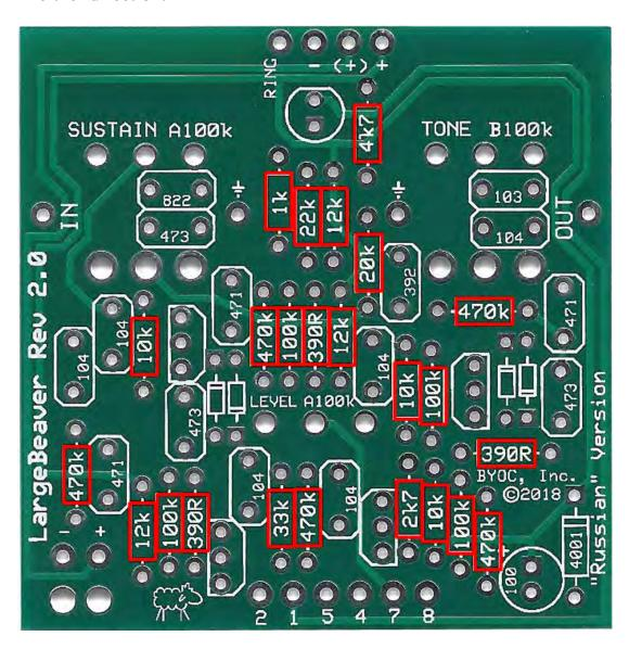
**Step 2**: Add the diodes. Be sure to match the end of the diodes with the stripe to the layout on the PCB. The striped end should go in the square solder pad.
