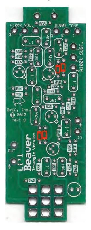
**Step 3:** Add the transistors. Be sure to match the tab side of the screenprint with the tab on the transistors.
