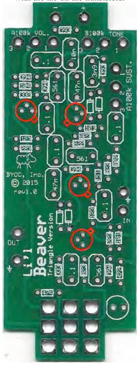
**Step 4:** Add the film and ceramic disc capacitors. These are non-polarized and can go in either direction. The ceramic disc capacitors are highlighted in yellow. Depending on the height of your ceramic disc capacitors, you may need to lay them on their side.
