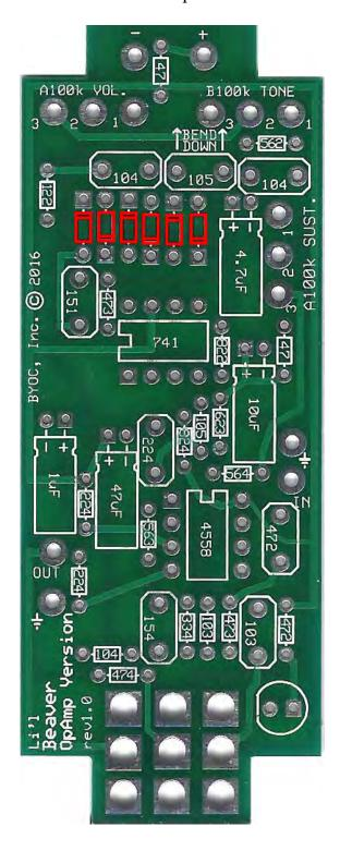
**Step 3:** Add the ICs. Be sure to orient them correctly. There may be a notch on the ICs between pins 1 and 8. Line that up with the screenprint on the PCB. If your ICs do not have a notch, look for a dot to indicate pin 1. Pin one on the PCB will be a square hole.
