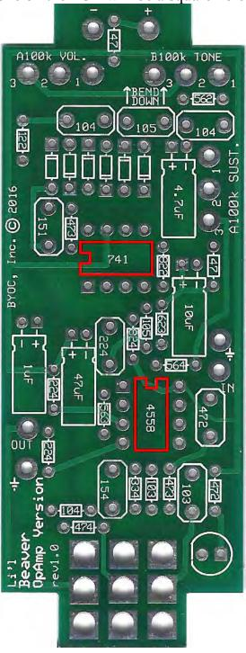
**Step 4:** Add the film and ceramic disc capacitors. These are non-polarized and can go in either direction. The ceramic disc capacitor is highlighted in yellow. Depending on the height of your ceramic disc capacitor, you may need to lay it on its side. The 1uF film cap highlighted in green should be bent to lie as flat as possible.
