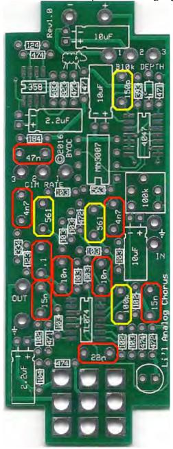
**Step 7:** Add the aluminum electrolytic capacitors. These ARE <u>polarized</u>, meaning there is a positive and negative end. The positive side will have a longer lead and goes in the square solder pad. The negative side will have a shorter lead and a stripe running along the body of the cap, and goes in the round solder pad. Before soldering, bend the capacitor so it is laying down like below.
