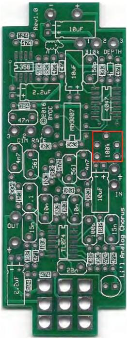
**How to set the trimpot:** After you finish your build, you will need to adjust the trimpot until you get the best chorus sound possible. First, set the trimpot to the middle of its rotation, and make slight adjustments until you hear the chorus effect. There will be a part of the sweep that will allow you to hear the chorus effect; within that window is where you want to set your trimpot. Use your ears to find the 'sweet spot'.
