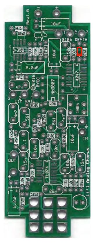
**Step 4:** Add the through-hole IC. Be sure to orient it correctly. There may be a notch on the IC between pins 1 and 8. Line that up with the screenprint on the PCB. If your IC does not have a notch, look for a dot to indicate pin 1. Pin one on the PCB will be a square hole.
