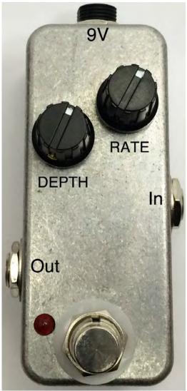
**DEPTH:** Control the intensity of the chorus effect. **RATE:** Controls the speed of the chorus effect.
