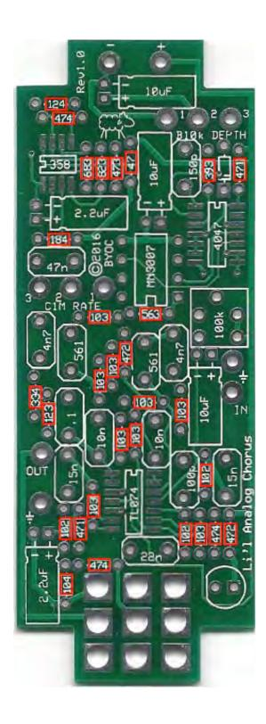
**Step 3**: Add the diode. Be sure to match the end of the diode with the stripe to the layout on the PCB. The striped end should go in the square solder pad.
