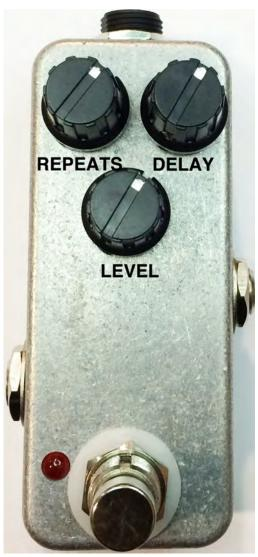
**LEVEL:** Controls overall output volume. **REPEATS:** Controls the amount of repeats.
