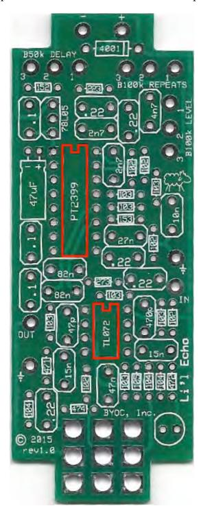
**Step 4:** Add the voltage regulator. Be sure to match the flat side of the transistor with the flat side on the screenprint.
