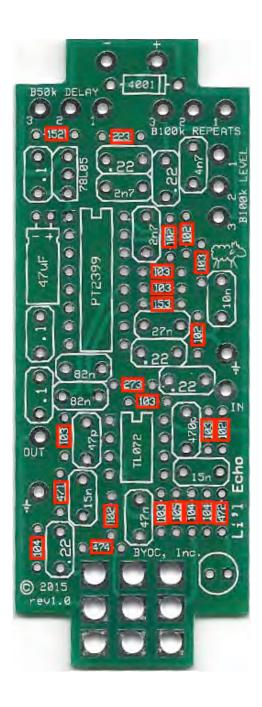
**Step 2**: Add the diode. Be sure to match the end of the diode with the stripe to the layout on the PCB. The striped end should go in the square solder pad.
