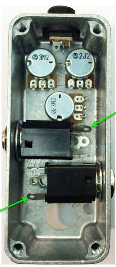
**Step 4:** Remove both nuts from the footswitch and mount the footswitch.
