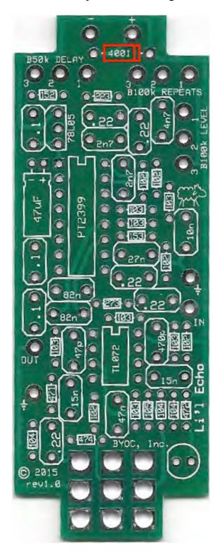
**Step 3:** Add the ICs. Be sure to orient them correctly. There may be a notch on the IC between the first pin and the last pin. Line that up with the screenprint on the PCB. If your IC does not have a notch, look for a dot to indicate pin 1. Pin one on the PCB will be a square hole.
