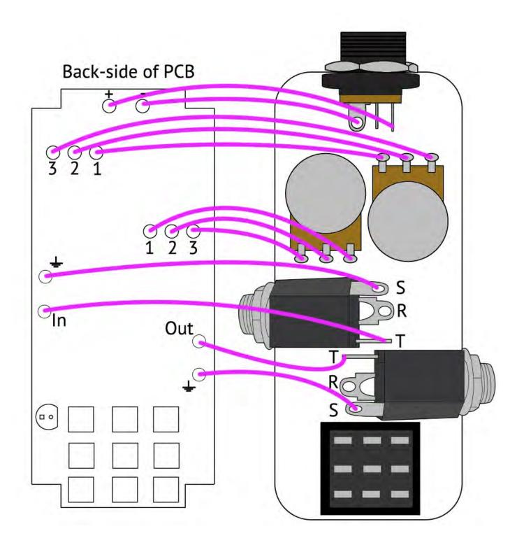
**Step 2:** Once the AC jack, potentiometer, and IN/OUT jacks are wired, insert the LED in its hole. **Insert the long lead into the square hole!!!** You might want to slightly bend the leads away from each other to keep them in the holes for now. DO NOT SOLDER YET
