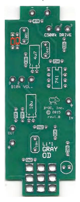
**Step 3:** Add the IC. Be sure to orient them correctly. There may be a notch on the IC between pins 1 and 8. Line that up with the screenprint on the PCB. If your IC does not have a notch, look for a dot to indicate pin 1. Pin one on the PCB will be a square hole.
