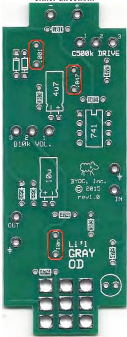
**Step 5:** Add the aluminum electrolytic capacitors. These ARE <u>polarized</u>, meaning there is a positive and negative end. The positive side will have a longer lead and goes in the square solder pad. The negative side will have a shorter lead and a stripe running along the body of the cap, and goes in the round solder pad. Before soldering, bend the capacitor so it is laying down like below
