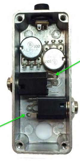
**Step 4:** Remove both nuts from the footswitch and mount the footswitch.
