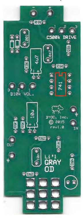
**Step 4:** Add the film capacitors. These are non-polarized and can go in either direction.
