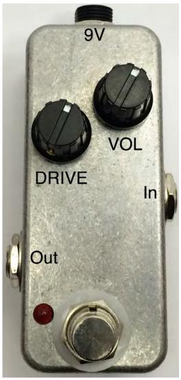
**VOL:** Controls overall output volume. **DRIVE:** Controls the amount of distortion.
