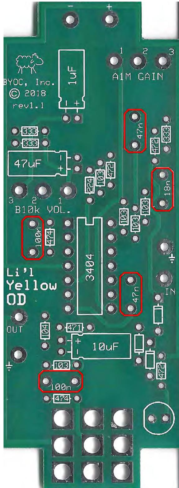
**Step 5:** Add the aluminum electrolytic capacitors. These ARE polarized, meaning there is a positive and negative end. The positive side will have a longer lead and goes in the square solder pad. The negative side will have a shorter lead and a stripe running along the body of the cap, and goes in the round solder pad. Before soldering, bend the capacitor so it is laying down like below.
