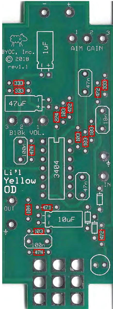
**Step 2:** Add the diodes. Be sure to match the end of the diodes with the stripe to the layout on the PCB. The striped end should go in the square solder pad.
