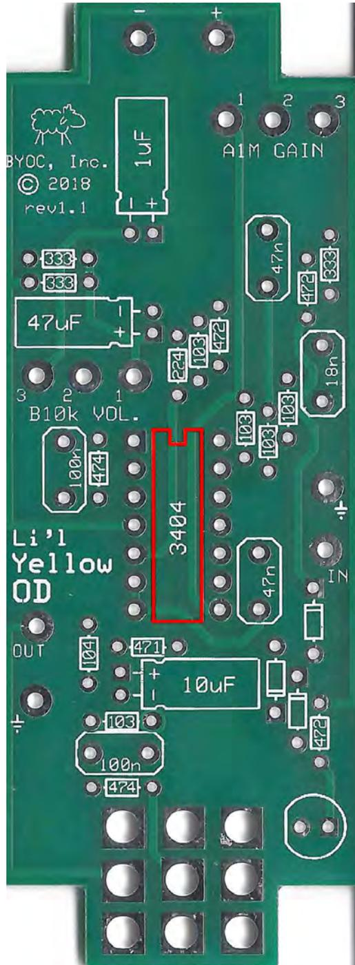
**Step 4:** Add the film capacitors. These are non-polarized and can go in either direction.
