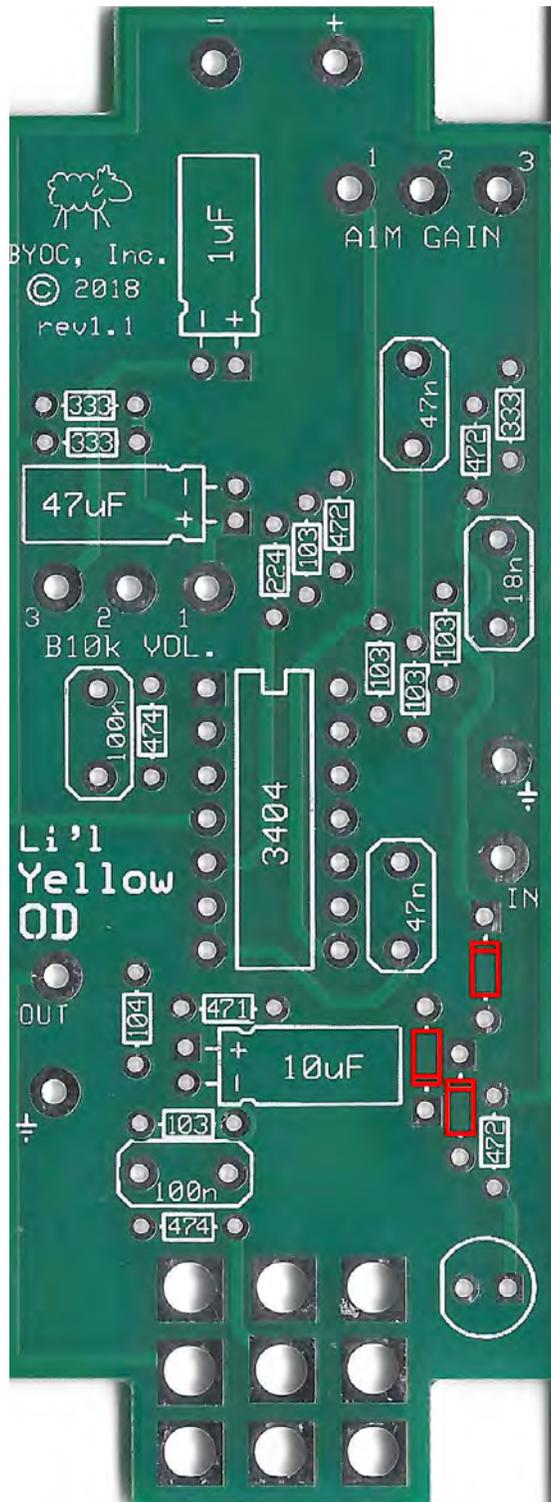
**Step 3:** Add the IC. Be sure to orient them correctly. There may be a notch on the IC between pins 1 and 14. Line that up with the screenprint on the PCB. If your IC does not have a notch, look for a dot to indicate pin 1. Pin one on the PCB will be a square hole.
