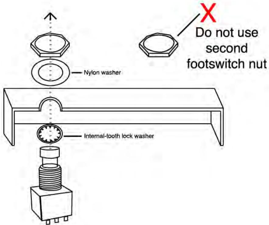
Orient the footswitch so that the flat sides of the solder lugs are like the diagram below.
