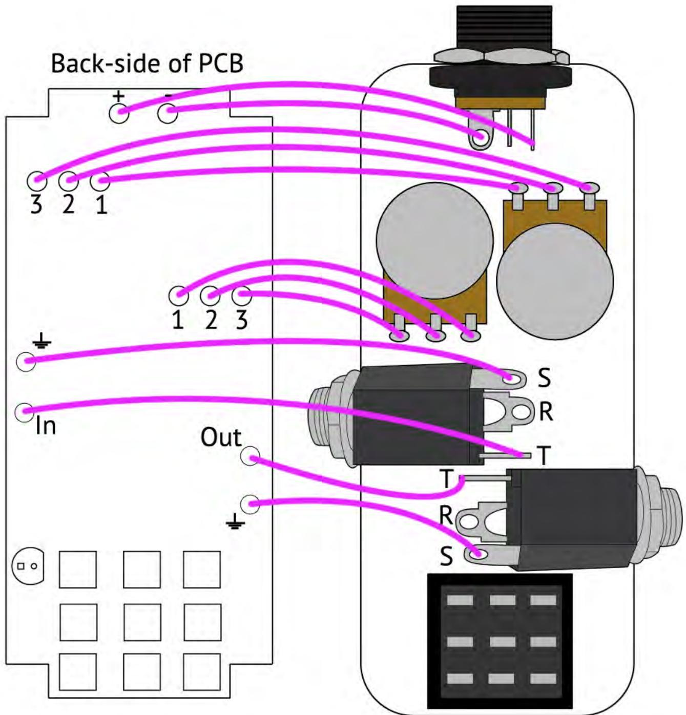
**Step 2:** Once the AC jack, potentiometer, and IN/OUT jacks are wired, insert the LED in its hole. **Insert the long lead into the square hole!!!** You might want to slightly bend the leads away from each other to keep them in the holes for now. DO NOT SOLDER YET
