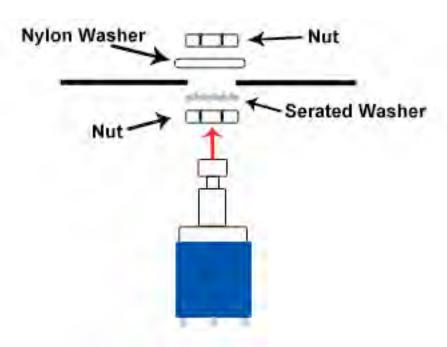
**Step 2:** Install the footswitch. Orient the footswitch so that the flat sides of the solder lugs are like the diagram below.
