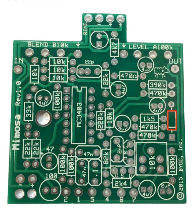
Step 3: Add the 14 pin socket. ONLY SOLDER THE SOCKET! NOT THE ACTUAL IC! This is a socket. The sockets get soldered to the PCB. The ICs get inserted into the sockets. The actual IC chip itself, never gets soldered. You will insert the IC into the socket after the entire pedal has been built. See page 25 for instructions on how to orient and install the ICs.
