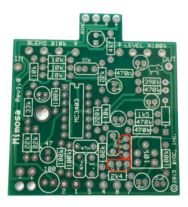
**Step 6:** Add the film and the ceramic disc capacitors. These are non-polarized so they can go in either direction. For the normal build, use the values listed on the PCB. To modify your Mimosa kit for use with a bass guitar, change the capacitors highlighted in blue to the .33u provided in your kit. **NOTE: Your kit may come with either a 22pf or 20pf ceramic disc capacitor based on availability.**
