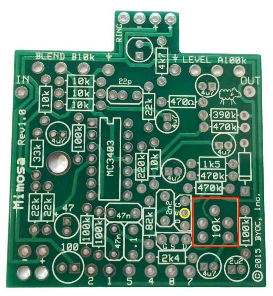
When you have finished building your mimosa kit, you will need to adjust the bias trimpot before the pedal will actually compress. You want to adjust the trimpot so that you get approximately 1.5-1.7V on the source of Q2. This would be the "S" eyelet highlighted in yellow.
