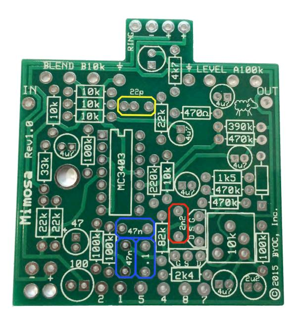
**Step 7:** Add the aluminum electrolytic capacitors. These ARE <u>polarized</u>, meaning there is a positive and negative end. The positive side will have a longer lead and goes in the square solder pad. The negative side will have a shorter lead and a stripe running along the body of the cap, and goes in the round solder pad.
