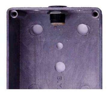
BEFORE CONTINUING, REMOVE THE DUST COVER FROM THE A100k DIST POTENTIOMETER. YOU MAY NEED TO MAKE A SLIT IN THE COVER TO RELIEVE ANY VACCUUM BETWEEN THE COVER AND THE POTENTIOMETER.
