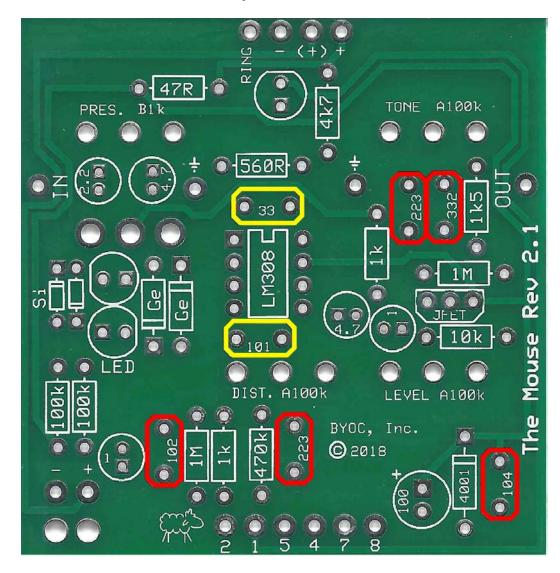
**Step 6:** Add the aluminum electrolytic capacitors. These ARE <u>polarized</u>, meaning there is a positive and negative end. The positive side will have a longer lead and goes in the square solder pad. The negative side will have a shorter lead and a stripe running along the body of the cap, and goes in the round solder pad.
