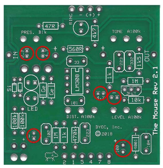
**Step 7:** Add the battery snap. Thread the leads into the strain relief holes first through the bottom side of the PCB. Then insert the leads into their respective solder pad hole on the top side of the PCB. The red lead goes in the + hole and the black lead goes in the – hole.
