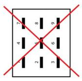
**Step 3a:** Make a jumper between lugs 3 & 6 from clippings from the resistors. Simply use your needle nose pliers to make a U shape & insert into lugs 3 & 6, then solder.
