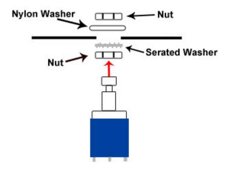
**Step 3:** Install the footswitch. Orient the footswitch so that the flat sides of the solder lugs are like the diagram below.
