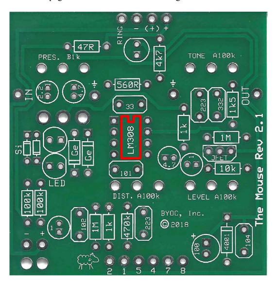
**Step 4:** Add the JFET. Orient it so that the flat side matches up with the flat side on the PCB layout.
