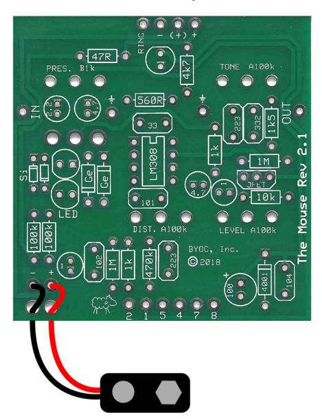
**Step 8:** Add wires to the IN, OUT, LED, POS, and the Ground eyelet located in the top of the board. Start by cutting 4 3.5" pieces of wire. Strip 1/4" off each end and tin the ends. Tinning means to apply some solder to the stripped ends of the wires. This keeps the strands from fraying and primes the wire for soldering. Load the wires in from the top and solder on the bottom of the PCB.
