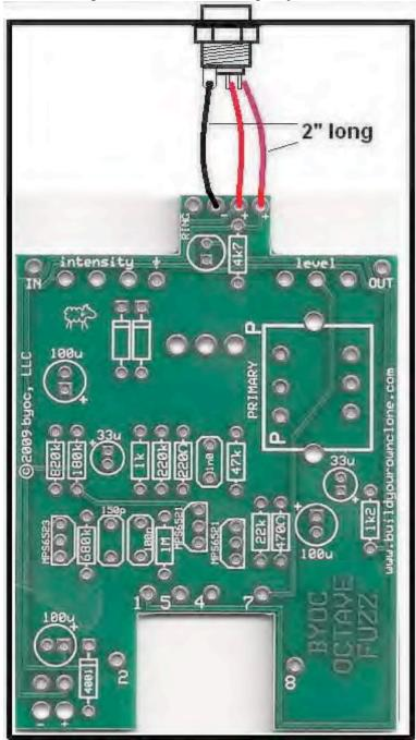
Step 2: Connect the TIP (negative) terminal of the DC adaptor jack to the "-" eyelet on the PCB with 2 inches of hook up wire. Connect the SLEEVE of the DC adaptor jack to the "+" eyelet on the far right side of the PCB with 2 inches of hook up wire. Connect the battery disconnect terminal of the DC adaptor jack to the "+" eyelet more towards the
