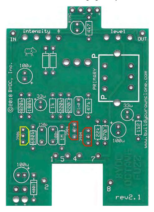
**STEP 5:** Add the aluminum electrolytic capacitors. These are polarized. The positive end will have a longer lead and should go in the square solder pad. The negative end will have a shorter lead with a black strip running down the body of the capacitor.
