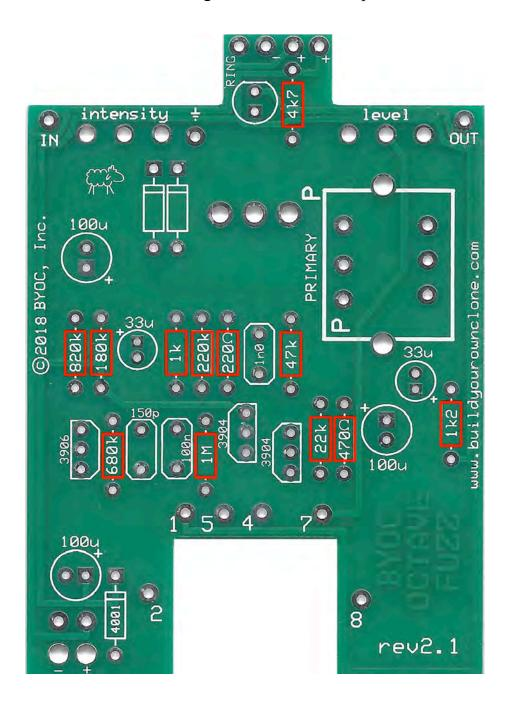
STEP 2: Add the diodes. The 1N4001 will be black with a silver stripe and is highlighted in yellow. The Germanium diodes will go in the spots highlighted in red. Be sure to match the end of the diode with the stripe to the layout on the PCB. The stripped end should go in the square solder pad. If your Germanium diodes have a white and gray stripe on either end, place the end with the gray stripe in the square hole. If your diodes have a single white dot, place the dot side into the round holes.
