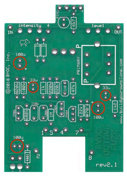
**STEP 6:** Add the transformer. A transformer has a primary and secondary side. The primary side will be labeled with a "P". Insert the transformer into the PCB so that the primary side matches the PCB.
