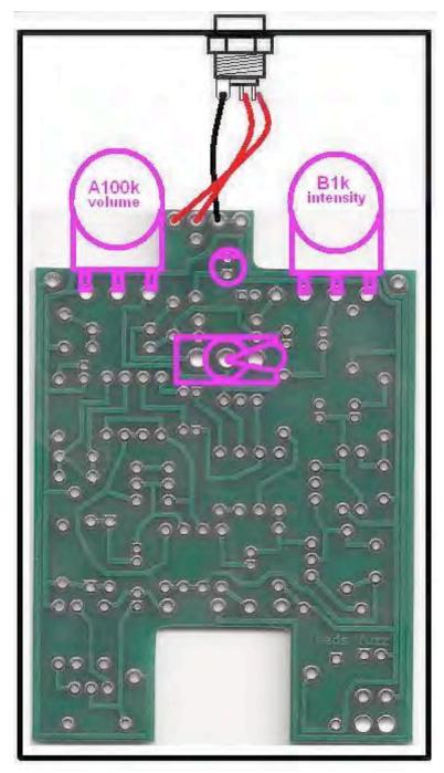
Step 3: Flip the PCB over so that the bottom or solder side is up. Insert the two potentiometers, the LED, and the toggle switch into the bottom side of the PCB. DO NOT SOLDER!!!There are only two ways in which the toggle switch can fit into the PCB. Either way is fine. The longer lead of the LED goes in the square solder pad hole and the shorter lead goes in the round solder pad hole.
