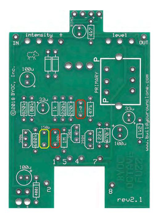
**STEP 4:** Add the transistors. Match the flat side of the transistor to the flat side of the layout on the PCB. The 2N3904 transistors are highlighted in red. The 2N3906 transistor is highlighted in yellow.
