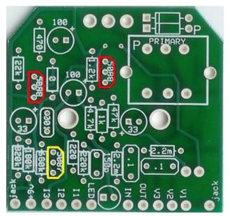
Step 3: Add the transistors. Make sure to match the flat side of the transistor up with the flat side on the PCB layout. Note that the slot for the 2N5087 is highlighted in yellow and the 2 2N5088's are highlighted in red.
