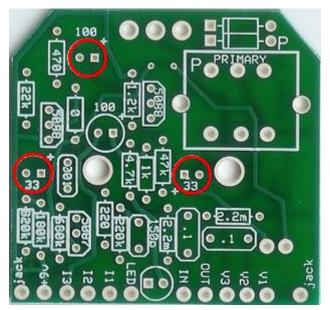
Step 5: Add the aluminum electrolytic capacitors. These are polarized. The positive end will have the longer lead and go into the square solder pad. The negative lead will be shorter and go into the round solder pad.
