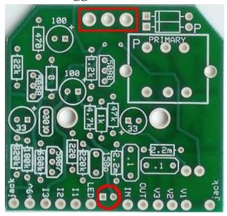
The toggle switch goes in the 3 eyelts at the top of the PCB. It does not matter which way you orientate the switch. If it fits in without having to bend the leads, then it will work just fine. The LED goes into the space at the bottom of the board between the "LED" and "IN" eyelets. The cathode of the LED (the shorter of the two leads, sometimes referred to as the negative end) goes in the square solder pad. The anode (longer positive lead) goes in the round solder pad.
