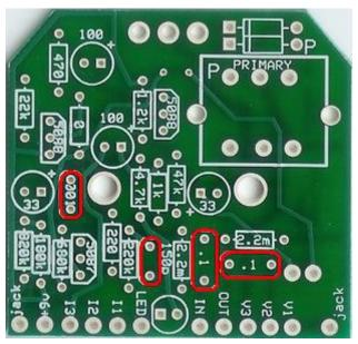
Step4: Add the 3 film capacitors and one ceramic disc capacitor. These are not polarized and can go in the PCB in either direction.
