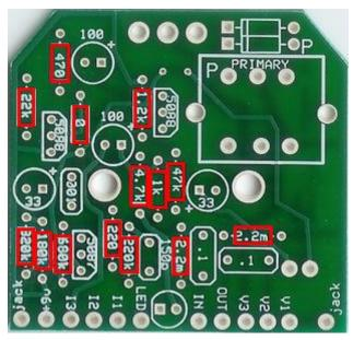
Step1: Add all resistors. Resistors are not polarized and can go in the PCB in either direction.
