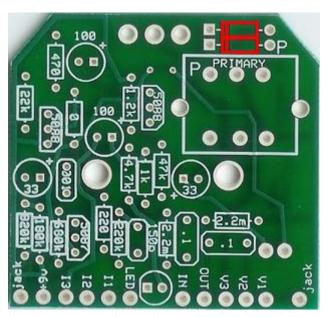
Step 2: Add the diodes. Make sure the end with the stripe (anode) matches the layout and goes in the square solder pad. Only add 2 diodes. Nothing goes in the 3rd diode slot.
