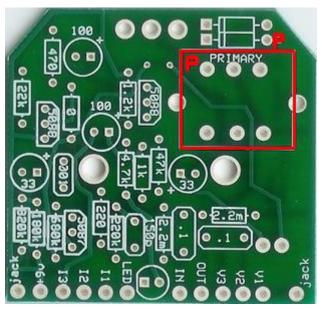
Step 6: Add the transformer. The primary side of the transformer will be marked with a "P". This side goes on the side of the PCB with a "P" on it.
