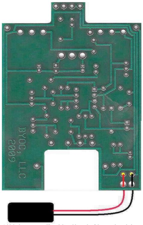
Step 8: Add the battery snap. Thread the solder ends of the snap through the under side of the strain relief holes. Insert the stripped ends of the battery snap wires into the topside of their respective solder pads. Solder on the bottom side where highlited in yellow. Remember the red wire goes in the "+" hole and the black wire goes in the "- "hole.
