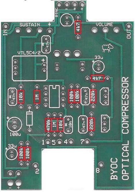
STEP 1: Add the resistors. Resistors are not polarized, so it does not matter which end goes in which solder pad.
