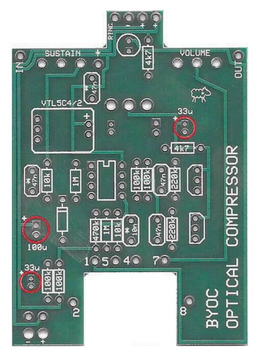
STEP 7: Add the aluminum electrolytic capacitors. These are polarized. The positive end will have a longer lead and should go in the square solder pad. The negative end will have a shorter lead with a black strip running down the body of the capacitor.
