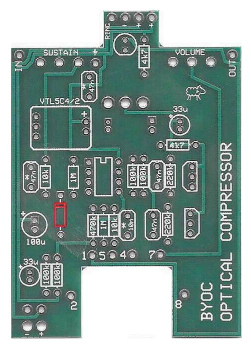
STEP 2: Add the diode. The 1N4001 will be black with a silver stripe. Be sure to matched the end of the diode with the stripe to the layout on the PCB. The stripped end should go in the square solder pad.
