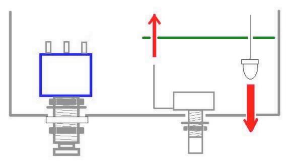
Step 5: Turn the entire pedal over so that the component side of the PCB if facing up. Lift the PCB up off the pots about 2mm just to make sure that the back of the PCB does not short out against that pots. Make sure the PCB is level and symetrically seated inside the enclosure.
