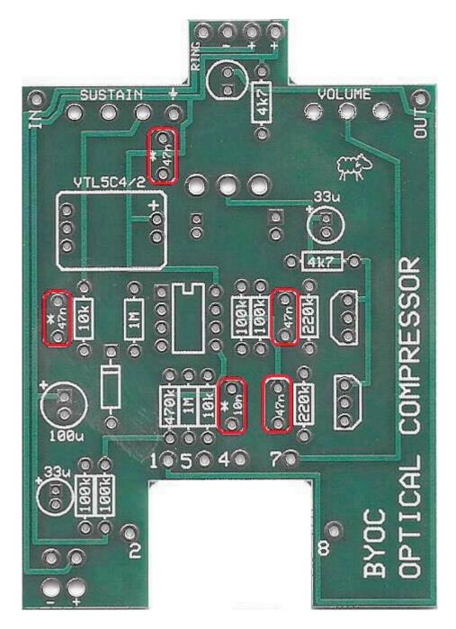
STEP 4: Add the film capacitors. These are not polarized so they can be inserted into the PCB in either direction. If you are building for use with bass guitar, you should use the .1uf(100n) capacitors in the places marked with an "\*".
