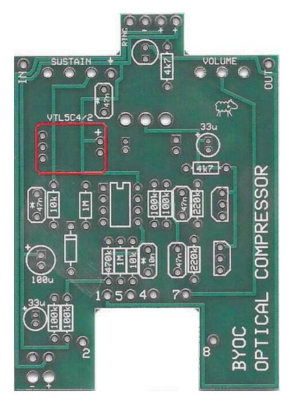
If your kit came with a VTL5C4/2(dual element with 5 leads): Orient the optocoupler so that the printed side is facing up and the "+" symbol on the optocoupler matches the "+" symbol on the PCB.
