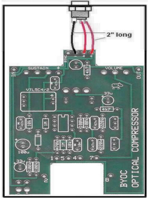
Step 2: Connect the TIP (negative) terminal of the DC adaptor jack to the "-" eyelet on the PCB with 2 inches of hook up wire. Connect the SLEEVE of the DC adaptor jack to the "+" eyelet on the far right side of the PCB with 2 inches of hook up wire. Connect the battery disconnect terminal of the DC adaptor jack to the "+" eyelet more towards the center of the PCB with 2" of hookup wire.
