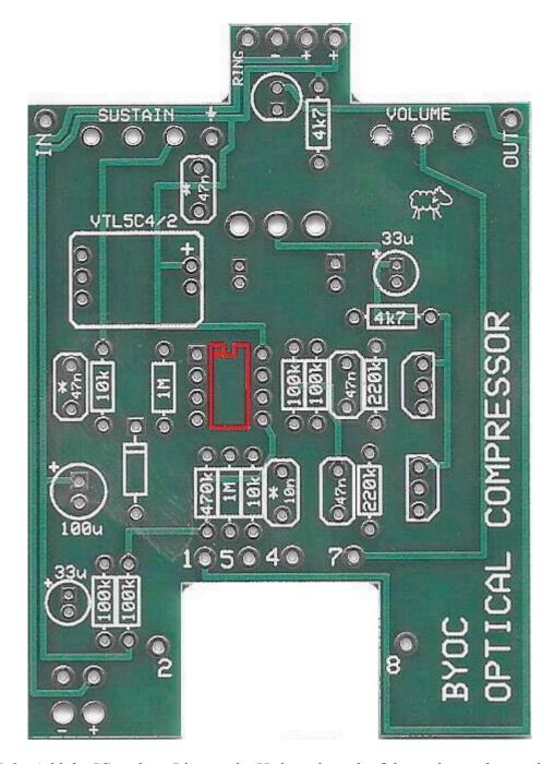
STEP 3: Add the IC socket. Line up the U shaped notch of the socket to the notch on the PCB layout. Solder only the IC socket to the PCB. Do not solder the actual IC. The IC inserts into the socket the same way you'd plug a vacuum tube into a socket. See page 21 for instructions on how to install the IC into the socket.
