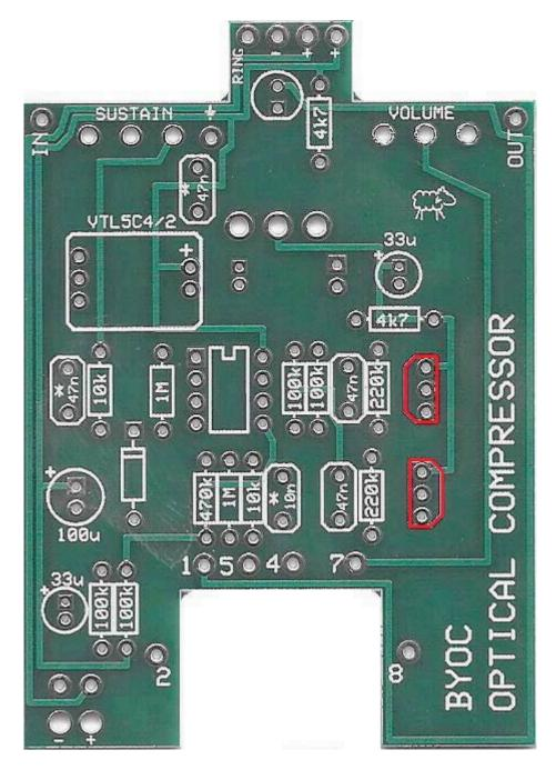
STEP 5: Add the transistors. Match the flat side of the transistor to the flat side of the layout on the PCB.
