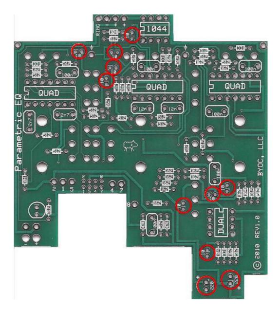
STEP 4: Add the aluminum electrolytic capacitors. These are polarized. The positive end will have a longer lead and should go in the square solder pad. The negative end will have a shorter lead with a black or white stripe running down the body of the capacitor.
