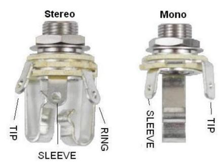
Step 1: Install the 1/4" jacks to the enclosure. Be sure to turn the OUT jack a 1/4 turn counter clockwise so that solder terminal for the tip does not short out against the enclosure.
