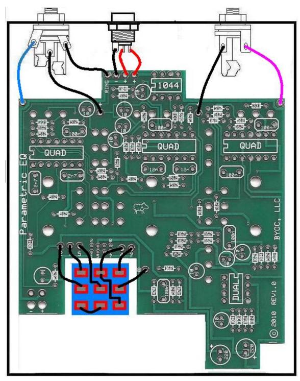
Step 3: Connect the pre stripped and tinned wires to the 1/4" jacks. Step 4:
