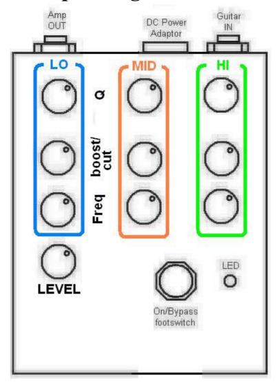
**Q**: Controls how wide or narrow the curve is of the frequency being boosted or cut. Clockwise produces a wider or lower Q. Counter-clockwise produces a narrower or higher Q.
