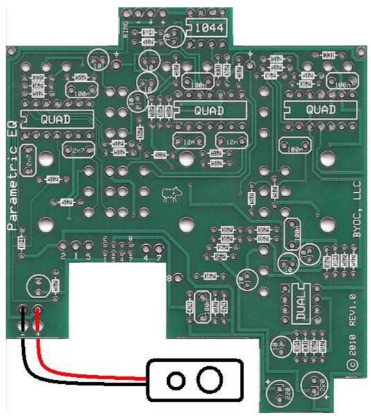
Step 5: Add the battery snap. Thread the solder ends of the battery snap into the strain relief holes from the bottom solderside of the PCB and out through the top. Insert the solder ends of the battery snap wires into the topside of their respective solder pads. Solder on the bottom side of the PCB. Remember the red wire goes in the "+" hole and the black wire goes in the "-" hole.
