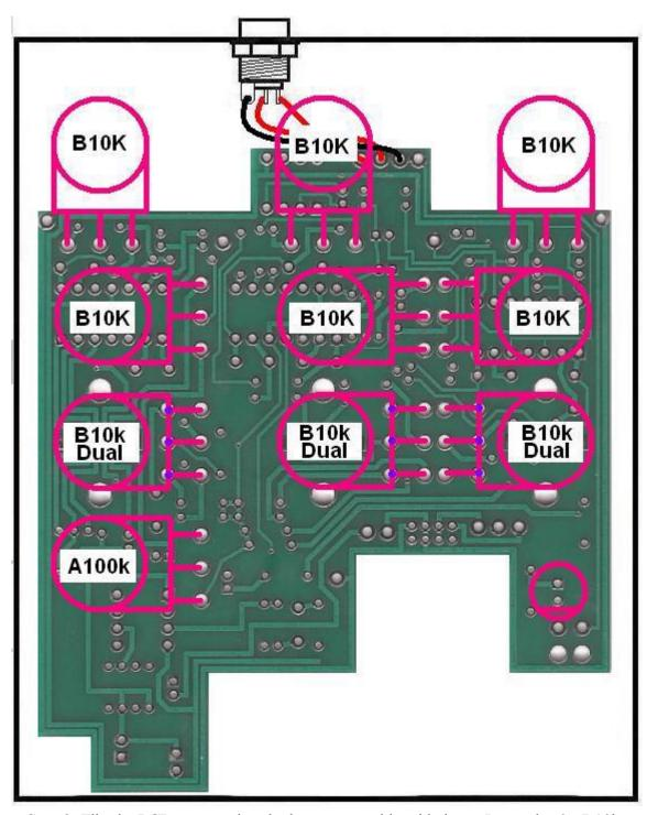
Step 3: Flip the PCB over so that the bottom or solder side is up. Insert the 6 x B10k (Boost/Cut & Q), 3 x Dual B10k (frequency), and 1 x A100K(level) potentiometers, and the LED into the bottom side of the PCB. DO NOT SOLDER ANYTHING YET!!! The LED will have one lead that is longer than the other. The longer lead goes in the hole with the square solder pad. The dual pots will have PCB snaps. You will never ever solder the dual pot snaps.
