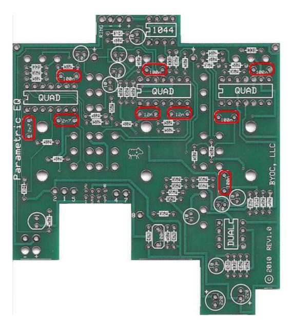
Step 3: Add the film capacitors. These are not polarized and can be inserted into the PCB either way.
