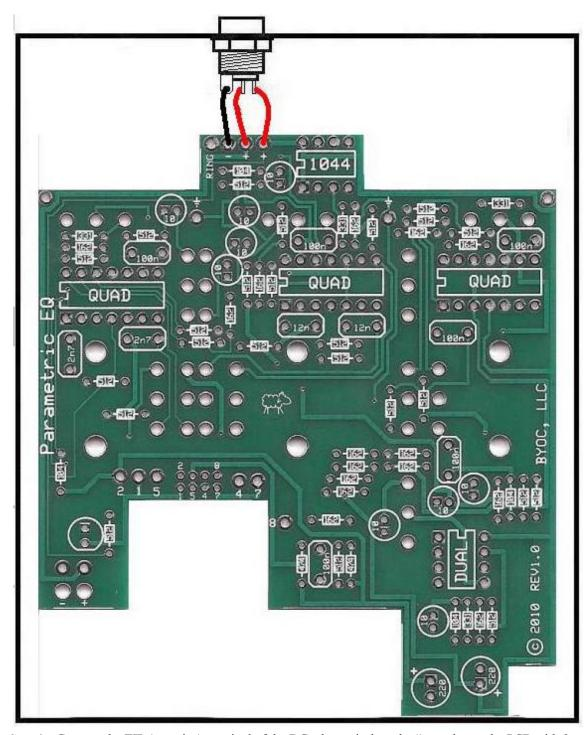
**Step 2:** Connect the TIP (negative) terminal of the DC adaptor jack to the "-" eyelet on the PCB with 2 inches of hook up wire. Connect the SLEEVE of the DC adaptor jack to the "+" eyelet on the far right side of the PCB with 2 inches of hook up wire. Connect the battery disconnect terminal of the DC adaptor jack to the "+" eyelet more towards the center of the PCB with 2" of hookup wire. Load the wires in from the bottom of the PCB and solder on the topside.
