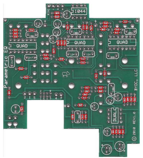
STEP 1: Add the resistors . Resistors are not polarized, so it does not matter which end goes in which solder pad. Note that your kit may come with either 5.1k or 5.11k for the 512 resistor spaces and 1.6k or 1.62k for the 162 resistors spaces.
