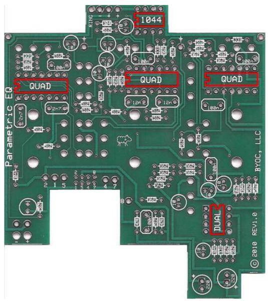
STEP 2: Add the 8 pin and 14 pin IC sockets. **ONLY SOLDER THE SOCKET! NOT THE ACTUAL IC!** These are sockets. The sockets get soldered to the PCB. The ICs get inserted into the sockets. The actual IC chips themselves, never get soldered. You will insert the ICs into the sockets after the entire pedal has been built.
