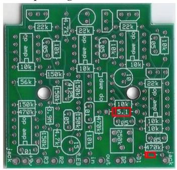
Step1: Add the diodes. The 1N914 goes in the smaller slot. The 5.1v Zener goes in the larger slot. make sure the black stripes line up with the layout.
