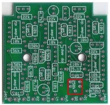
Step 4: Add the 250k trimpot. There should be only one what that this component will fit in the board. When you are finished with your phaser kit, you will need to adjust this trimpot till you hear a phasing sound. Your phaser may work the very first time you plug it in, but still adjust this pot for the best sounding phase.
