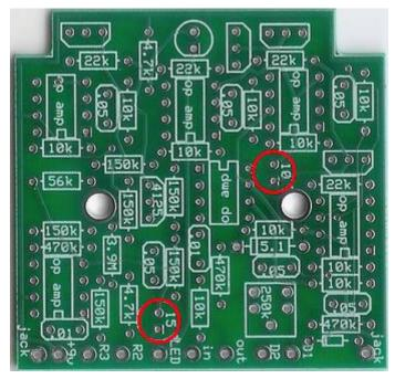
Step 7: Add the electrolytic caps. NOTE your kit may not come with a 15uf cap. If it doesn't have a 15uf cap it should have two 10uf caps. The 15uf cap can be replaced with the 10uf. Electrolytic caps are polarized. The positive end will have a longer lead and should go in the square solder pad.
