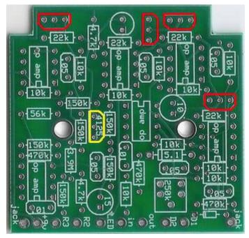
Step 5: Add the transistors. Make sure you orientate them so that the flat sides match up with the layout. The 2N5952 are highlighted in red. The 2N4125 is highlighted in yellow.
