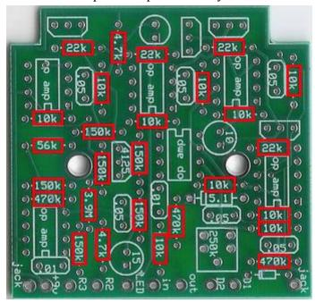
Step 2: Add the resistors. Resistors are not polarized so this means you can put them in either direction.
