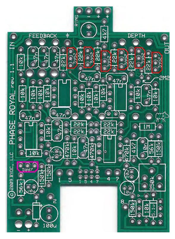
**Step 6:** Add the Transistors. The six 2N5952 JFETs go in the spots highlighted in red. The 2N5087 goes in the spot highlighted in pink. Be sure to orient the transistors so that the flat side of the transistor body matches up with the flat side on the PCB layout.
