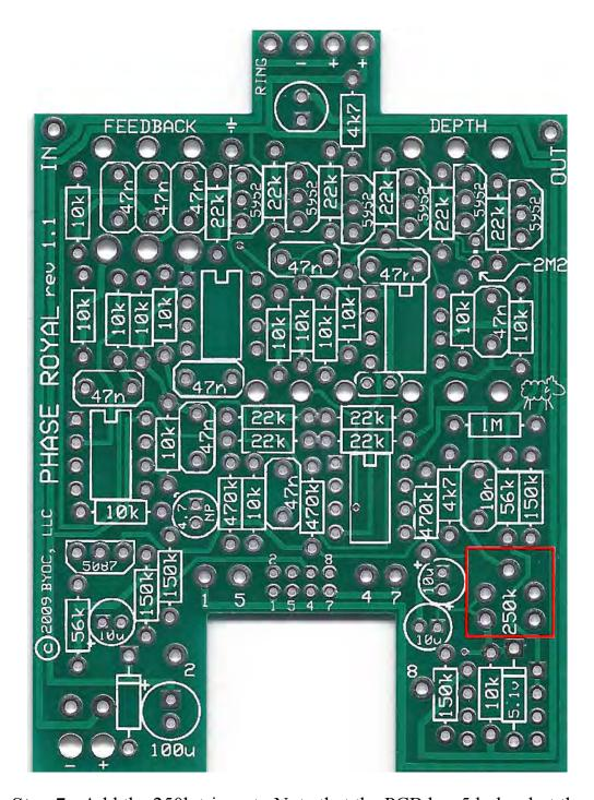
**Step 7:** Add the 250k trimpot. Note that the PCB has 5 holes, but the actual trimpot itself will only have 3 leads. This is so that the PCB can accommodate a variety of different makes and model of trimpots. There should only be one way in which the trim pot provided with your kit fits easily into the PCB.
