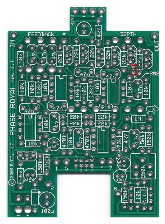
**Step 3:** Add the 2.2M (2M2) resistor. Stand it on end. Insert one end into one of the eyelets highlighted in red. Bend the other end and insert it into the other eyelet highlighted in red. See pictures below for examples.
