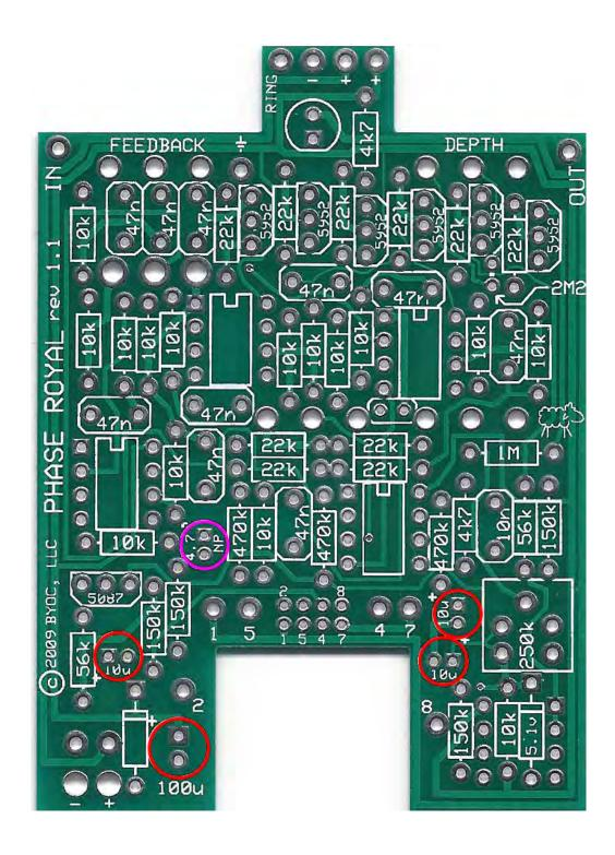
**STEP 8:** Add the aluminum electrolytic capacitors. These are polarized. The positive end will have a longer lead and should go in the square solder pad. The negative end will have a shorter lead with a black strip running down the body of the capacitor. The 4.7uF highlighted in pink is non-polarized which means you can insert it in any direction.
