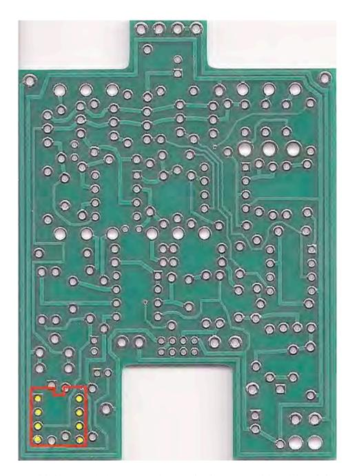
**Step 9:** Add the remaining IC socket to the bottom solder side of the PCB. Be sure to orient the socket so that the notch matches the outline in the diagram above.
