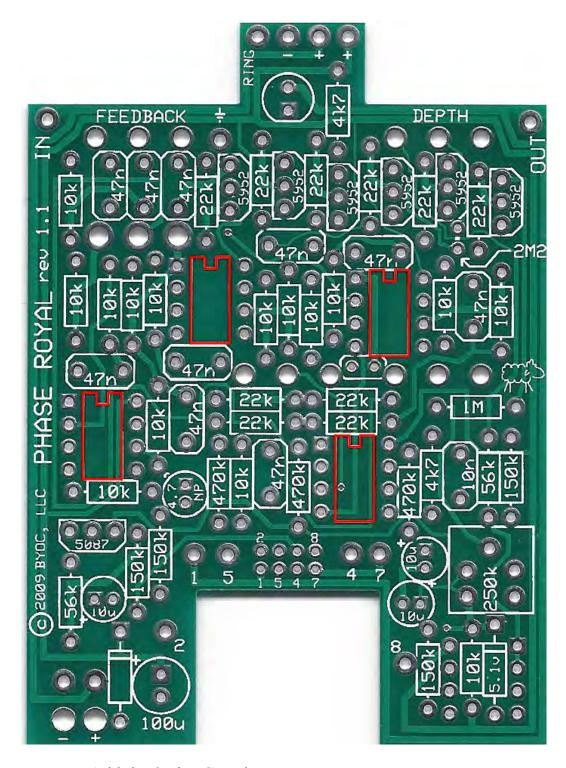
STEP 4: Add the 8 pin IC sockets. ONLY SOLDER THE SOCKET!
