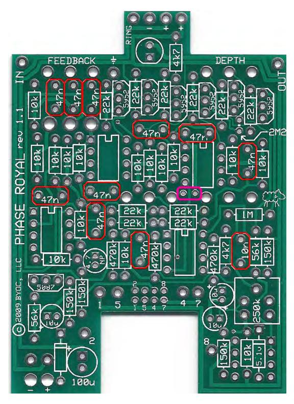
**STEP 5:** Add the film and ceramic capacitors. These capacitors are non-polarized, so you can insert them into the PCB either way. The capacitor highlighted in pink is the ceramic disc.
