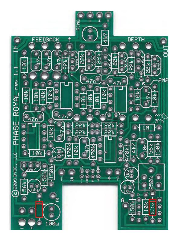
**Step 2:** Add the diodes. Be sure to match the end of the diode wit the stripes to the layout on the PCB. The striped end should go in the square solder pad. The Black Silicon 1n4001 diode goes in the space with no markings. The orange glass 1n4733 5.1v Zener diode goes in the spot marked '5.1v'.
