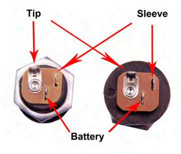
**Step 6:** Connect the TIP (negative) terminal of the DC adapter jack to the eyelet on the PCB labeled "-". Connect the SLEEVE of the DC adapter jack to the eyelet on the PCB labeled "+" farthest to the right. Connect the battery disconnect terminal of the DC adapter jack to the second eyelet on the PCB labeled "+" located in the middle of the other two eyelets.
