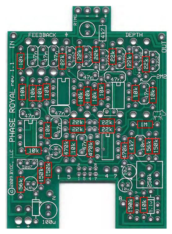
STEP 1: Add the resistors. Resistors are not polarized, so it does not matter which end goes in which solder pad. Do not add the 2.2M (2M2) resistor yet.
