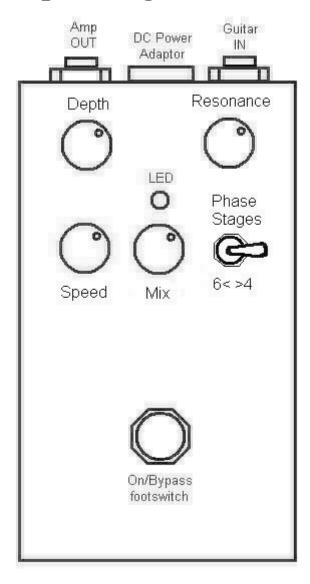
DEPTH: Sometimes called Width or Intensity. Controls intensity of the actual phase shifting.
