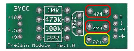
**Step 4:** Add the transistor. Be sure to match the flat side of the transistor with the flat side of the PCB layout.
