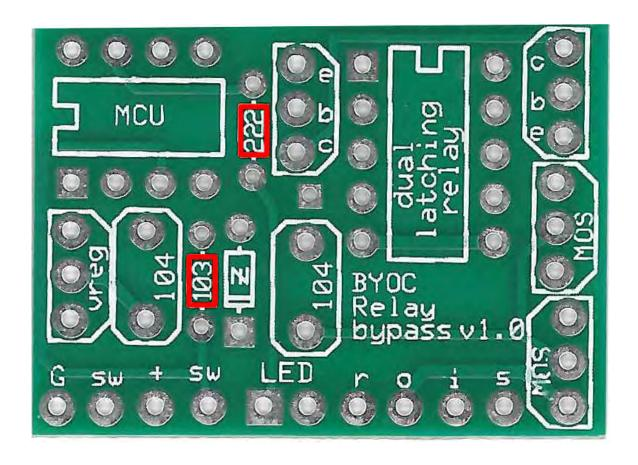
**Step 2:** Add the Zener Diode. Be sure to match the stripped end of the diode with the stripe on the PCB screenprint.
