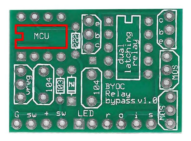
**Step 4:** Add the Relay. There will be a stripe on one end of the relay to indicate pins 1 and 10. Install it so that the stripe is above the notch on the screenprint.
