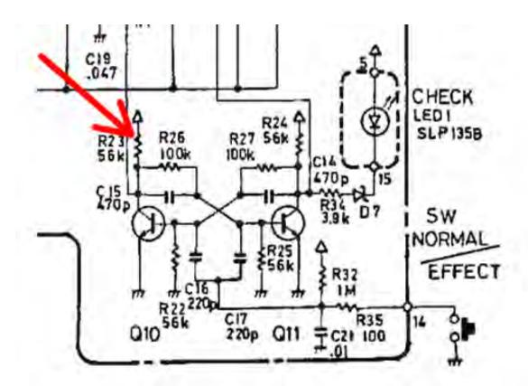
The red arrow points to the resistor you need to remove to prepare the BOSS flip-flop circuit. This is an excerpt taken from a BOSS CS-1 factory schematic. Here, the resistor designator is R23. In your pedal, the resistor designator may be something else. But it will most likely be a 56k resistor and circuit will be identical.
