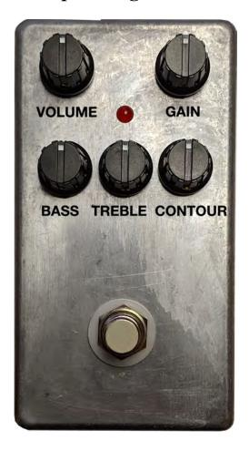
**VOLUME:** This controls the volume of the pedal. **GAIN:** This controls the amount of distortion.
