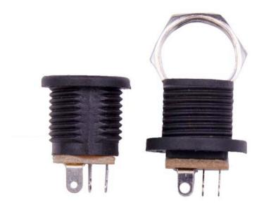
**Step 1:** Mount the AC adapter jack to the enclosure. Your kit may come with either an external thread or internal thread. Don't get confused by this. They still function exactly the same. You just thread the external nut on the outside and the internal nut on the inside. The picture below is of an internal nut jack.
