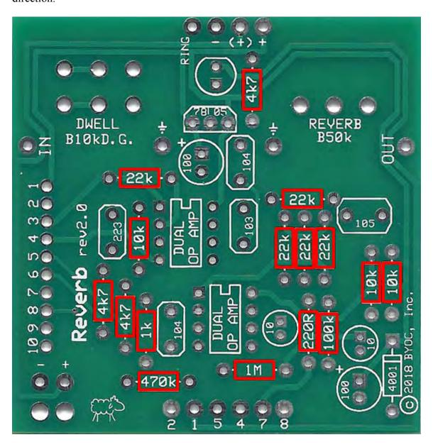
**Step 2**: Add the 1n4001 diode. Be sure to match the end of the diode with the stripe to the layout on the PCB. The striped end should go in the square solder pad.
