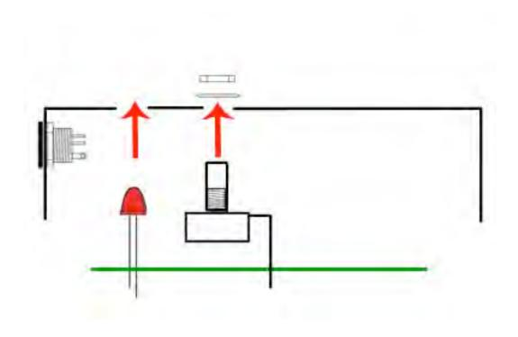
**Step 3:** Hold the PCB in one hand so that the component side of the PCB is in the palm of your hand and the bottom side with the pots, toggle switch and LED is facing up. Now use your other hand to guide the predrilled enclosure onto the PCB assembly so that the pots and LED all go into their respective holes. Once the PCB assembly is in place, secure it by screwing on the washers and nuts for the pots. Only tighten them with your fingers. You do not want them very tight yet.
