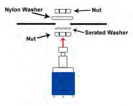
**Step 2:** Install the footswitch. Orient the footswitch so that the flat sides of the solder lugs are like the diagram below.
