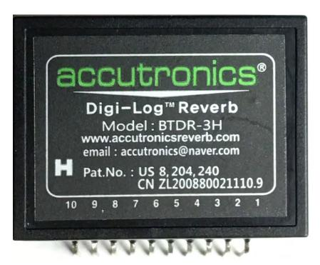
Once you've done this, install and solder the Reverb Module to the underside of the PCB. There is only one way the Module will fit in the PCB if you are inserting it into the underside. Solder the 10 pins on the topside of the PCB.
