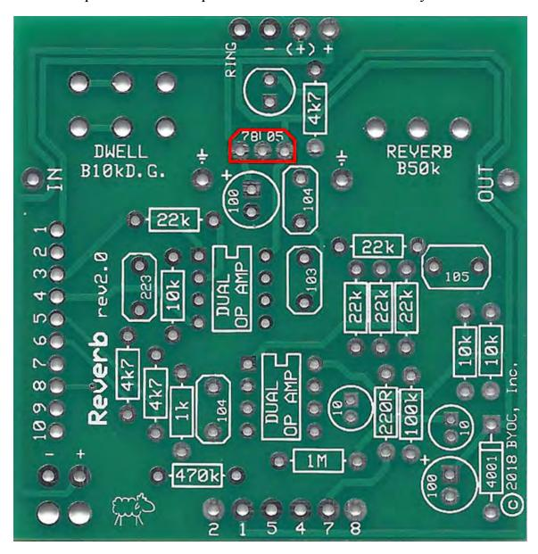
**Step 6:** Add the aluminum electrolytic capacitors. These are <u>polarized</u>, meaning there is a positive and negative end. The positive side will have a longer lead and goes in the square solder pad. The negative side will have a shorter lead and a stripe running along the body of the cap, and goes in the round solder pad.
