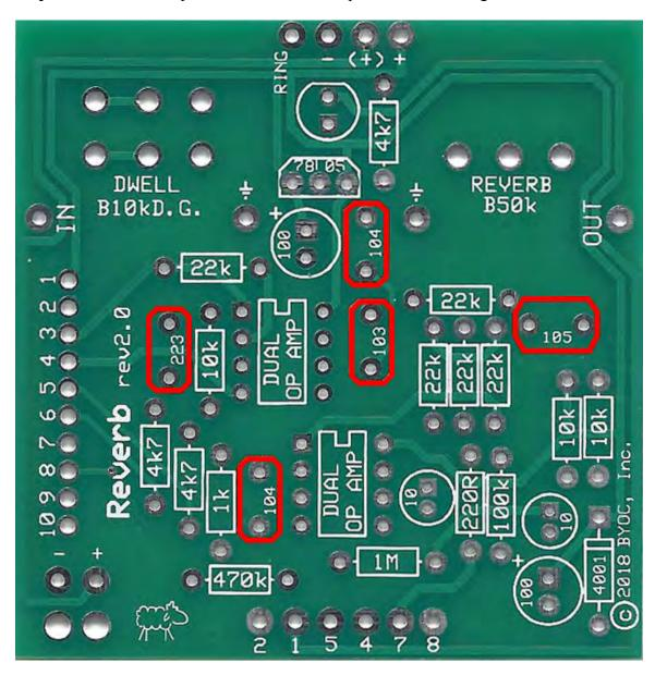
**Step 5**: Add the voltage regulator. Insert it into the PCB so that the flat side of the component matches up with the flat side of the PCB layout.
