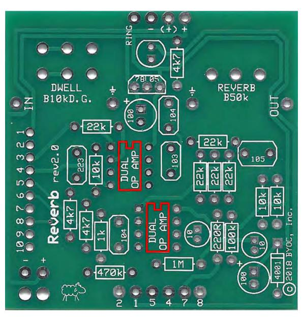
Step 4: Add the film capacitors. These are non-polarized so it can go in either direction.
