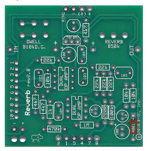
Step 3: Add the 8 pin IC sockets. ONLY SOLDER THE SOCKETS!
