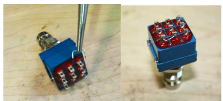
• Cut a 1.5" piece of wire. Strip 1/8" of one end. Strip 1/2" off the other end. Tin both ends. This will be used to connect lug/eyelet 4. The longer stripped end will be used to jumper lug 4 to 9.
