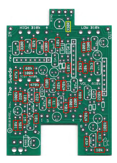
Note: The 120 Ohm and 10k resistors have the same color bands, just reversed. Find the 120 Ohm resistor with your multimeter before soldering any 10k resistors. One of the brown bands is the tolerance band, and will be slightly offset on the 120 Ohm relative to the 10k resistors.
