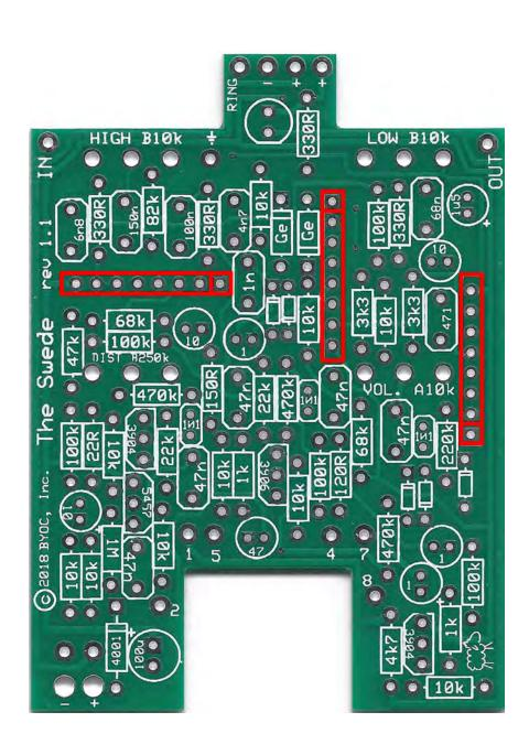
**Step 4:** Add the transistors. Be sure to match the flat side of the transistor with the flat side of the transistor on PCB layout. The **red** transistors are 3904, the **yellow** transistor is 3906, and the **green** transistor is 5457.
