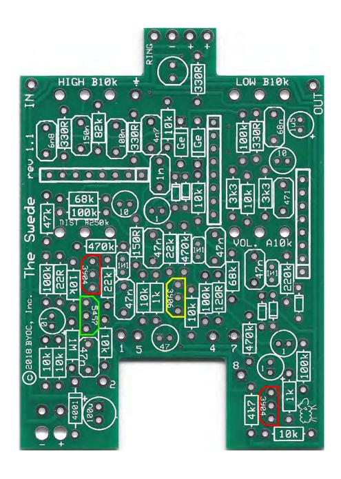
**Step 6:** Add the film (red outline) and the ceramic disc (yellow outline) capacitors. These are non-polarized so they can go in either direction.
