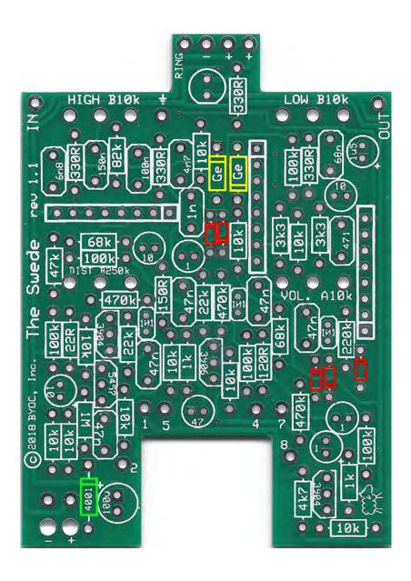
Step 3: Add the 8 pin sockets. ONLY SOLDER THE SOCKET! NOT THE ACTUAL IC! This is a socket. The sockets get soldered to the PCB. The ICs get inserted into the sockets. The actual IC chip itself, never gets soldered. You will insert the IC into the socket after the entire pedal has been built. See page 27 for instructions on how to orient and install the ICs.
