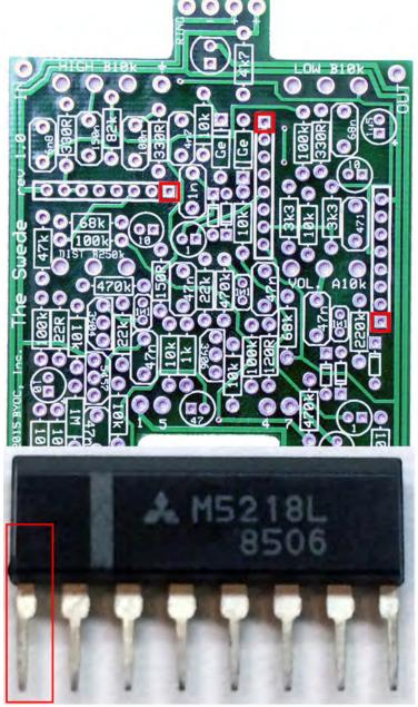
The red areas indicate pin 1 of the M5218L IC, and the location of those pins on the PCB.
