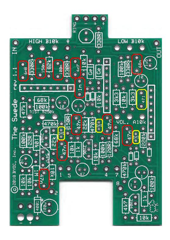
**Step 7:** Add the aluminum electrolytic capacitors. These ARE <u>polarized</u>, meaning there is a positive and negative end. The positive side will have a longer lead and goes in the square solder pad. The negative side will have a shorter lead and a stripe running along the body of the cap, and goes in the round solder pad.
