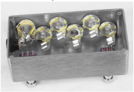
Step 3: Install the Jacks. Notice how all of the mono jacks are rotated slightly. This is to insure that there are no bare metal contacts touching any other bare metal contacts. Use common sense when installing the jacks. If you see contacts from two jacks touching. Rotate one or both slightly so that there is no contact. Once you have all the jacks in place, use a 3/8" wrench or socket to tighten.
