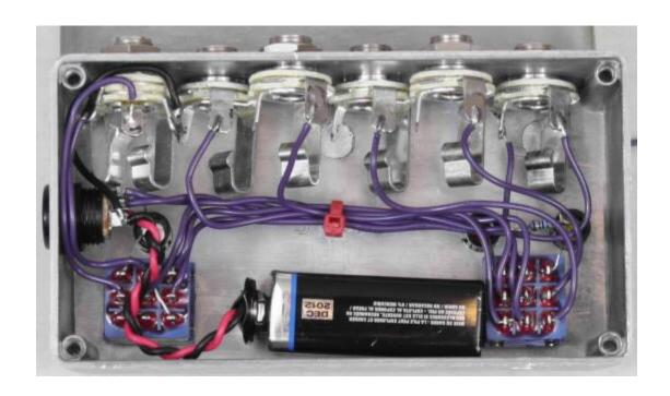
Step 9: Test your bypass looper. If everything works the way it's supposed to, use the cable tie to bundle your wiring. If it's not working correctly, trouble shoot your build and getting working properly before you tie the wiring.
