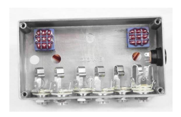
Step 4: Install the footswitches. Notice that the A/B footswitch is rotated a 1/4 turn. Below is the numbering system used to differentiate the solder lugs on a 3PDT footswitch.
