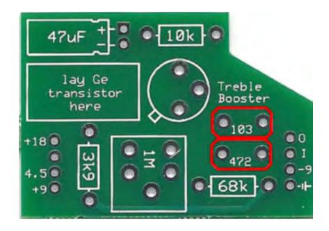
**Step 5:** Add the electrolytic capacitor. Before soldering, bend the capacitor so it lays flat along the screenprint outline.
