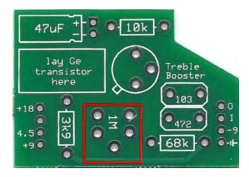
**Step 3:** Add the transistor socket. Be sure to match the tab on the socket with the tab outline on the PCB screenprint. You will lay the transistor on the board after you have placed it in the socket.
