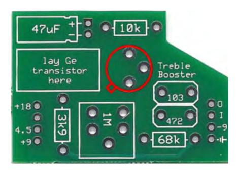
**Step 4:** Add the Film caps. These are not polarized and can be placed in either direction.
