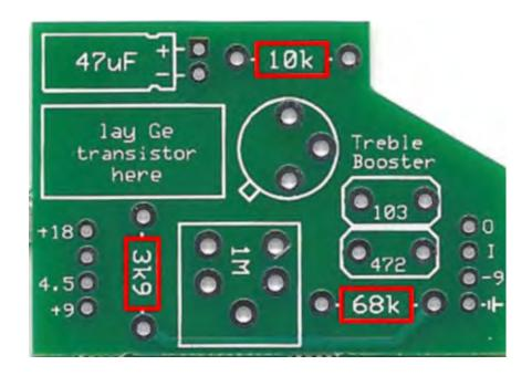
**Step 2:** Add the Trimpot. The PCB has 5 holes. This is to accommodate various sizes of trimpots. You will only be soldering three of them.
