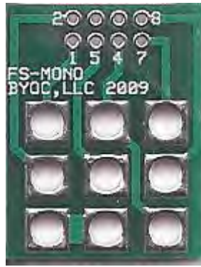
Top Side of Footswitch PCB
